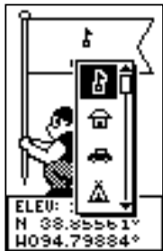
The Mark Waypoint Page allows you to change the symbol for the waypoint.
