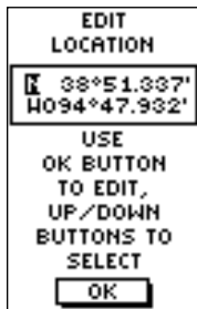
The EDIT LOCATION Page displays on-screen instructions explaining how to edit the waypoint location.
