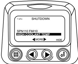
3. To acknowledge and "Hide" the fault and return to the single or four parameter display touch the "Enter Button"
