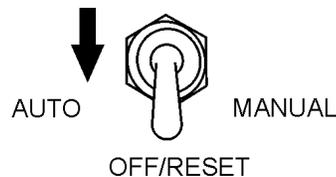
**Figure 56. MPEC Control Switch (Off/Reset)**
