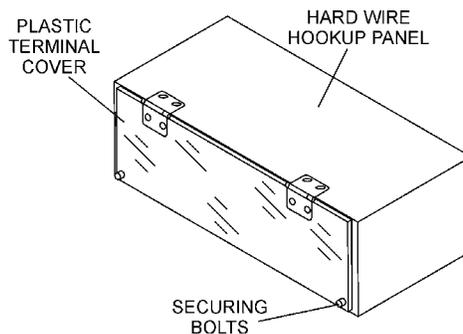
Figure 11. Plastic Face Plate (Output Terminal Lugs)
