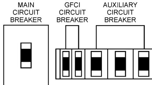
**Figure 54. Main, GFCI and Load Circuit Breakers Off**
