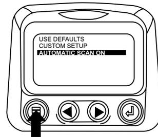
19. Touch the “Menu Button” to exit the Main menu and return to the engine parameter display.
