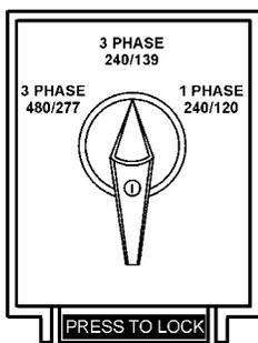
Figure 15. Voltage Selector Switch
