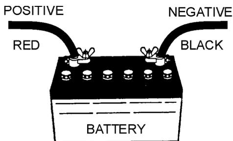
Figure 36. Battery Connections
