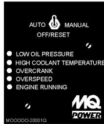
has a vertical row of status LED's (inset), that when lit, indicate that an engine malfunction (fault) has been detected. When a fault has been detected the engine controller will evaluate the fault and all major faults will shutdown the generator. During cranking cycle, the ECU will attempt to crank the engine for 10 seconds before disengaging.
