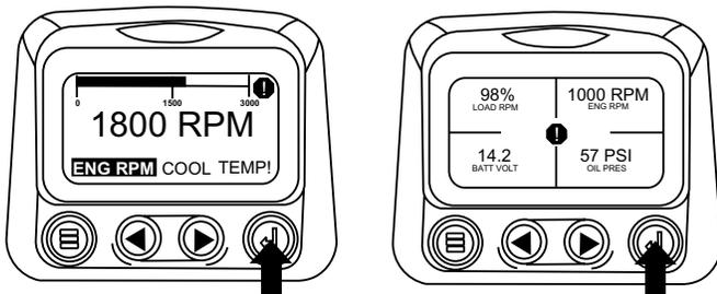
5. Touching the "Enter Button" once again will hide the fault and return the screen to the single or four parameter display.
