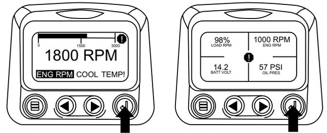
2. The main menu will pop up on the display. Use the "Arrow Buttons" to scroll through the menu until the "Adjust Backlight" is highlighted.
