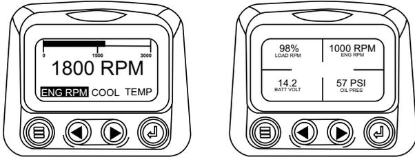
2. When the diagnostic display receives a severe fault code from an engine control unit the single or four parameter screen will be replaced with the "Shutdown" message.
