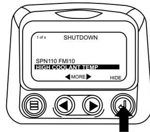
6. The Single or Four parameter screen will display the fault icon until the fault condition is corrected. NOTE: Ignoring active fault codes could result in severe engine damage.
