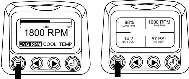
2. The main menu will pop up on the display. Use the arrow buttons to scroll through the menu until the “Select Units” is highlighted.
