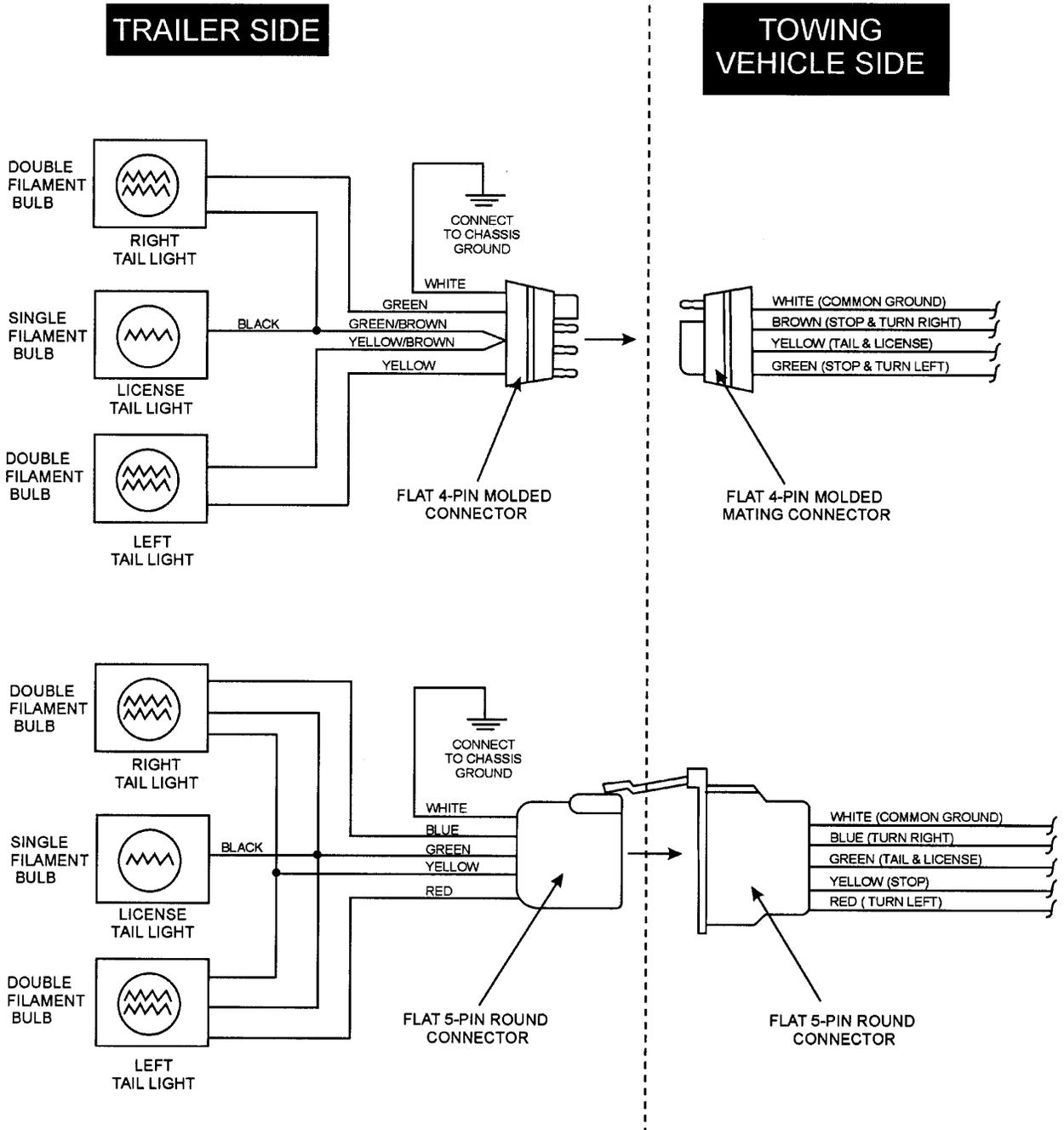
Figure 63. Trailer/Towing Vehicle Wiring Diagram
