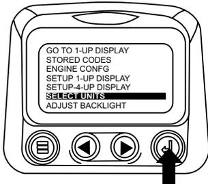
4. Use the arrows to highlight the desired units. “English” for imperial units i.e. PSI, °F or Metric kPa, Metric Bar for IS units i.e. kPa, Bar, “C”.
