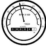
**Figure 51. Engine Tachometer Gauge**
