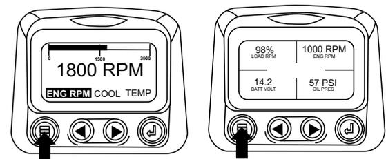
2. The main menu will pop up on the display. Use the “Arrow Buttons” to scroll through the menu until the “Setup 1-up Display” is highlighted.
