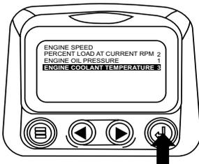
14. Continue to scroll and select additional parameters for the custom 1-up Display. Touch the “Menu Button” at any time to return to the “Custom Setup” menu.
