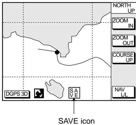
*Figure 7-9 SAVE icon appearance on the plotter display*
