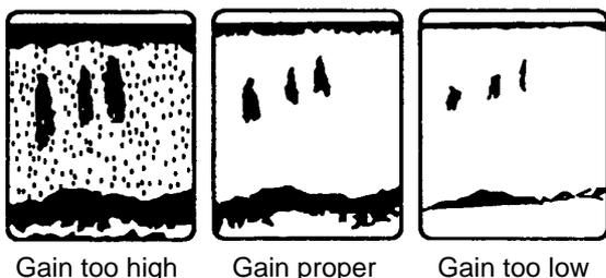
Figure 2-17 Examples of proper and improper gain
