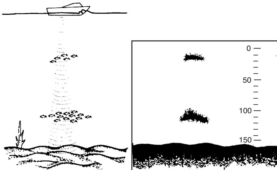
Figure 2-1 Underwater conditions and video sounder display
