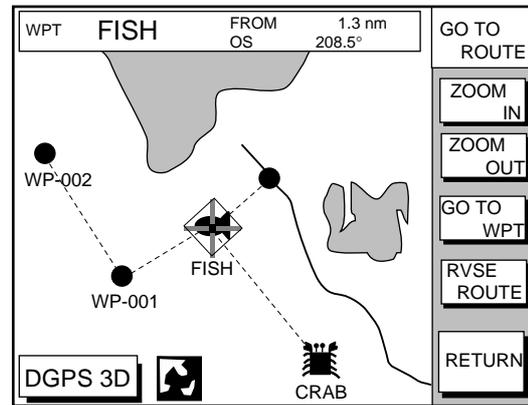
Figure 8-6 Plotter display, route selected as destination
