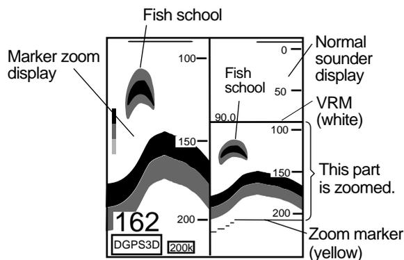
Figure 2-7 Marker-zoom display plus normal sounder display
