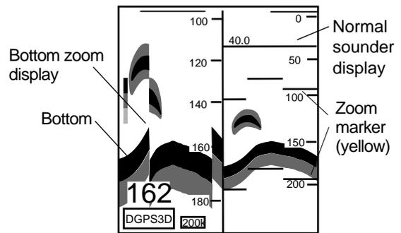
Figure 2-8 Bottom-zoom display plus normal sounder display
