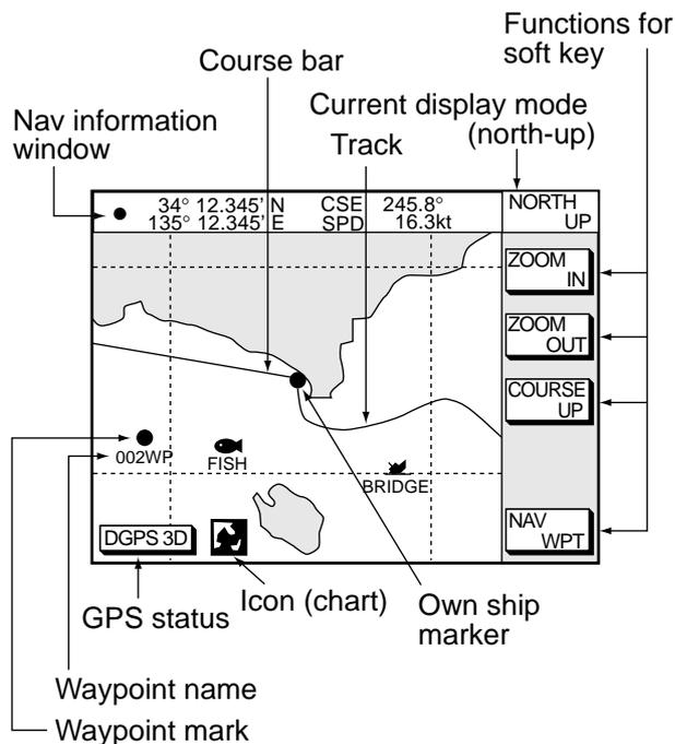
Figure 3-1 Plotter display, north-up mode
