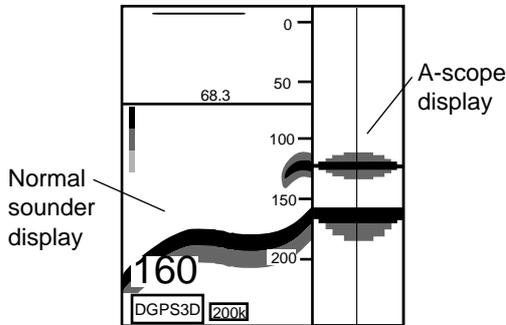
Figure 2-10 A-scope display plus normal sounder display
