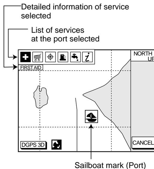
Figure 3-8 Plotter display showing Nav-Charts™ port service display
