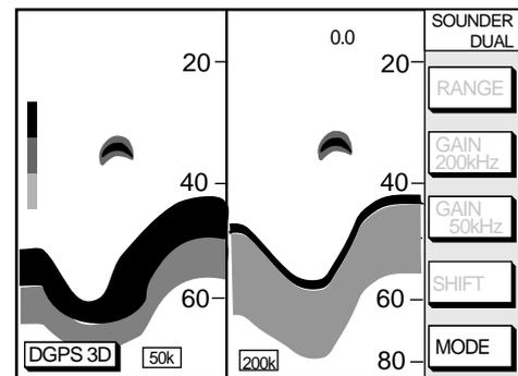
Figure 2-13 Dual-frequency display
