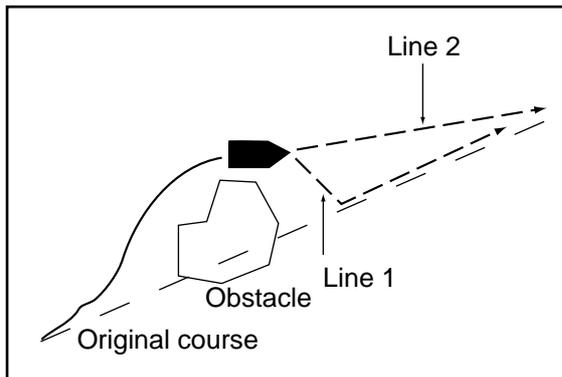
Figure 8-7 Example of when to restart navigation
