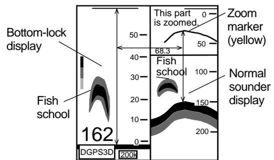
Figure 2-9 Bottom-lock display plus normal sounder display
