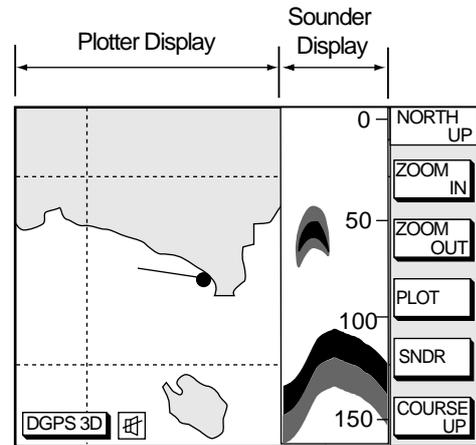
Figure 2-12 Plotter/Sounder display
