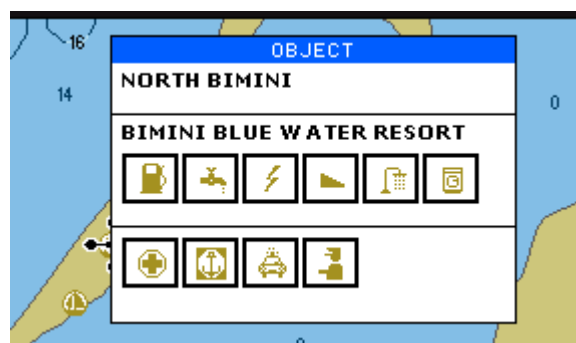
Sample filling station, service marks
