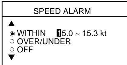
*Figure 8-9 Speed alarm window*
