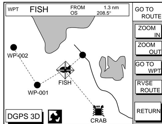
Figure 7-6 Plotter display, route selected as destination
