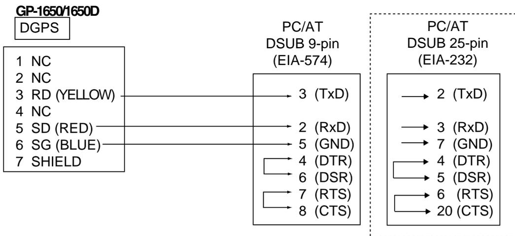
Figure 10-17 Connection of GP-1650D/GP-1650 to PC
