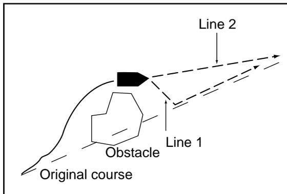
Figure 7-7 Example of when to restart navigation
