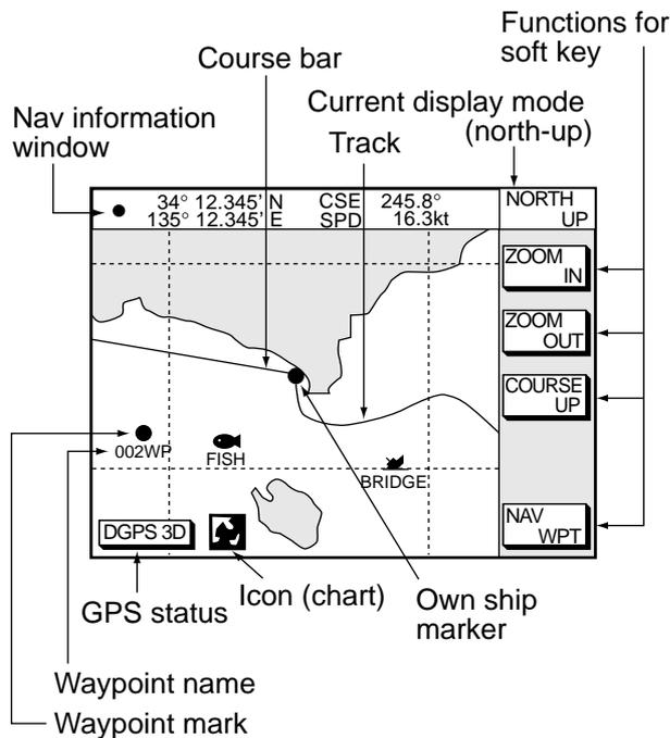
Figure 2-1 Plotter display, north-up mode
