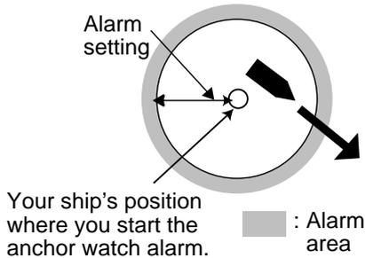
Figure 8-5 How the anchor watch alarm works
