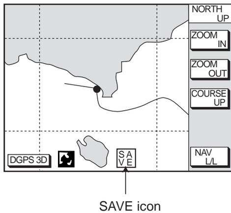
*Figure 6-9 SAVE icon appearance on the plotter display*
