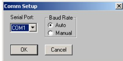
**Setup:** Opens the Comm Setup Window, shown to the left. Select the **Serial Port** to which the sensor is connected from the drop-down list. Then select **Auto** (the program determines the baud rate on its own) or **Manual** (you then enter the baud rate) for the Baud Rate entry.
