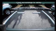
The Rear View Camera allows you to see blind spots behind a vehicle by automatically projecting its rear view on the display whenever the gear is in reverse.
