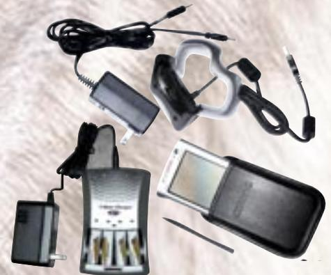
Wolf Receiver System includes a carrying case, stylus, ac adaptor, 8 AA Ni-MH batteries, fast-charger, USB cradle and iPAQ PDA with expansion pack sled.
