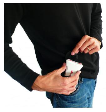
Alternatively, LonerGPS may be worn in a pocket, however the mobile worker should ensure that the logo side of the enclosure should face away from their body.
