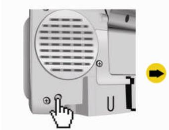
Execute the soft reset by the pressing the Reset button as shown left: **Lightly press the button once.**
