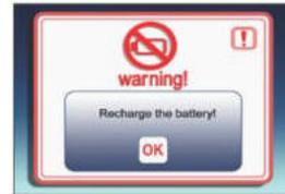
When you fail to recharge the battery after the warning window is displayed, the system is forcibly switched to the power-saving mode. Refer to 'Power Mode and Battery Recharging.'
