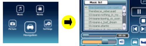
3. Pressing the menu button on the front of the body returns the system to the menu program from the current program.
