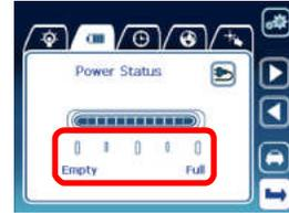
In the battery-powered mode, the Power Status icon is displayed as 'Battery', and the Battery Remainder Power meter indicates the current remaining Power Status icon power in the battery.
