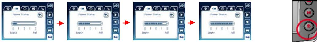
When the battery is fully charged, the Battery Remainder Power meter does not move, but is kept at the 'Full' condition. The Power button on the body lights green.
