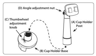
Step 2. Place the universal cup holder mount into the designated cup holder in the vehicle. Adjust the thumbwheel adjuster (C) to expand or close the cup holder prongs to fit in the cup holder.
