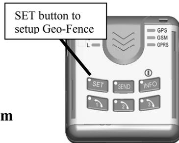
Press the SET button to set a 200 m Geo-fence around the device.
