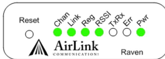
**Tx** (transmit) and **Rx** (receive) - Lights will flash as data is transferred to and from the modem on the network.
