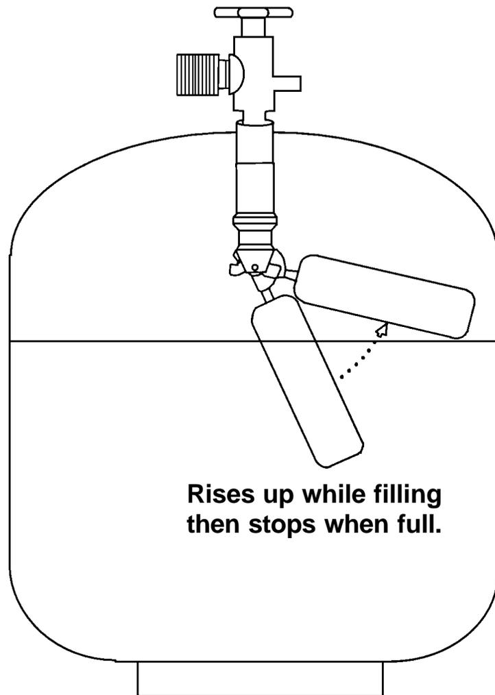
**⚠ WARNING!** Do not exchange the LP Gas cylinder unless the exchange LP cylinder is equipped with an OPD. Otherwise you will lose the OPD (Overfilling Prevention Device) feature. If there is not an LP cylinder available for exchange equipped with an OPD, we recommend that you have your cylinder filled at an authorized LP gas dealer by a qualified attendant.
