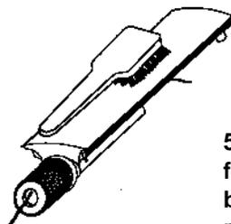
5. Use a pipe cleaner to clear obstructions from all burner holes. A brass wire brush can be used on the burner surfaces to remove corrosion.
