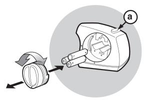
The Weber Grill Out "Handle Light has a "Tilt Sensor": Lid up - ON / Lid Closed - OFF. The power button (a) activates or deactivates the "Tilt Sensor." For daytime use, deactivate the sensor by pressing power button (a).
