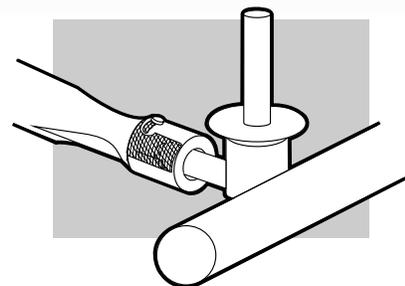
⚠ **WARNING:** After reinstalling the gas lines, they should be leak checked with a soap and water solution before using the barbecue. (See Step: "Check for gas leaks.")
