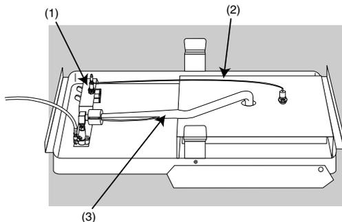
Make sure wire is connected between igniter and electrode. Check that igniter lock nut is tight.
