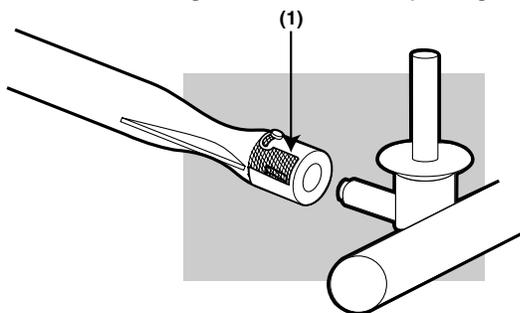
We recommend that you inspect the Spider/Insect screens at least once a year. (See Section “Annual Maintenance”.) Also inspect and clean the the Spider/Insect screens if any of the following symptoms should ever occur:
