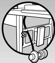
We utilize various LP tank manufacturers. Some of the tanks have differing top collar assemblies. (The top collar is the metal protective ring around the valve.) One series of tanks mount with the valve facing front. The other tanks mount with the valve facing away from the fuel scale. These types of tanks are illustrated below.
