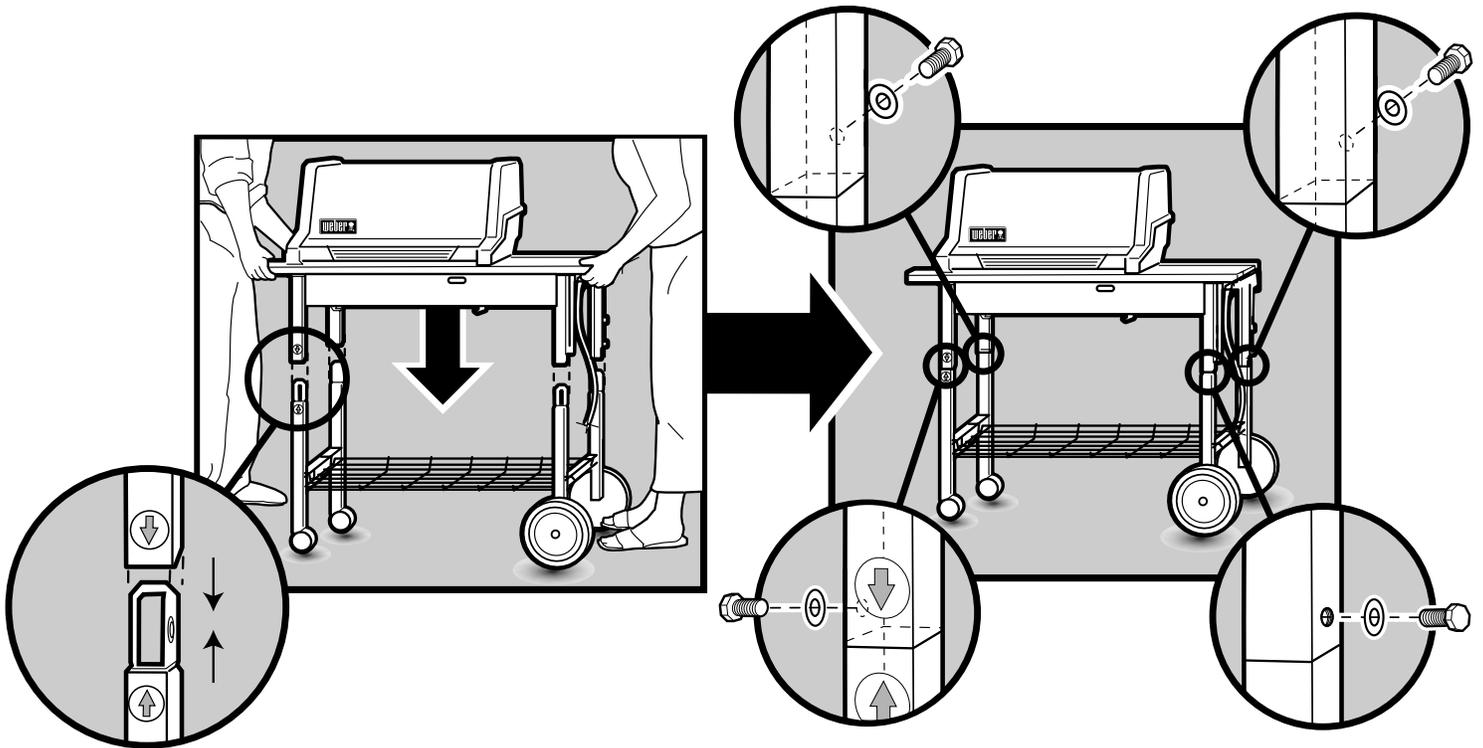
• Install bolts at indicated locations. Use supplied tool to tighten. Recheck each bolt for tightness with a 7/16" open end wrench.
