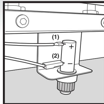
Place corresponding control knobs down onto the valve stems. From the underside of the control panel, replace the two wires (1, 2) of each igniter.
