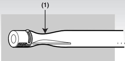
The burner tube air shutter is fitted with a stainless steel screen(1) to prevent spiders and other insects access to the burner tubes through the air shutter openings.
