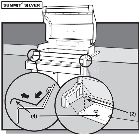
Remove the Front Panel by sliding the panel up and out of the slots.
