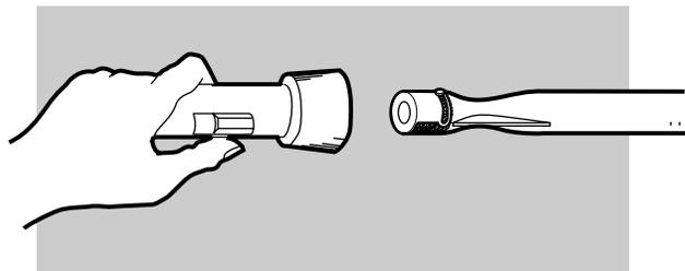
Clean the inside of the burners with a wire (a straightened-out coat hanger will work). Check and clean the air shutter opening at the ends of the burners. Check and clean the valve orifices at the base of the valves. Use a Steel bristle brush to clean outside of burners. This is to make sure all the burner ports are fully open.
