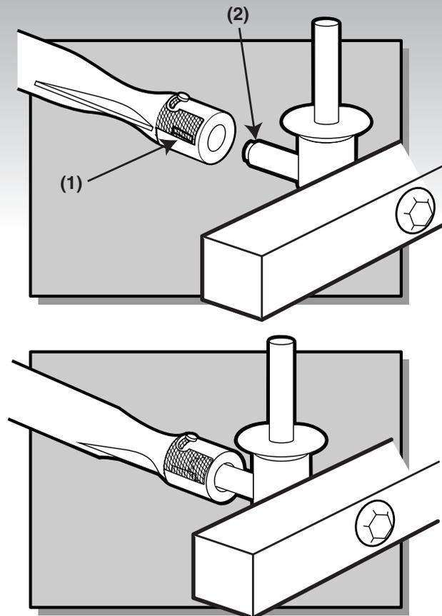
Check proper assembly before fastening manifold in place.
