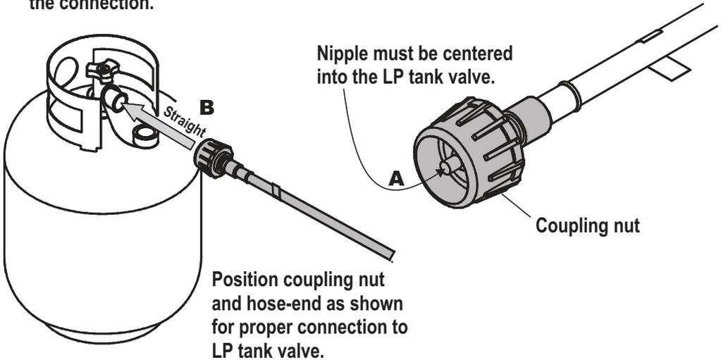
6. Turn the coupling nut clockwise to tighten to a full solid stop. The hose-end will seal on the back-check feature in the LP tank valve, resulting in some resistance. **An additional one-half to three quarters turn is required to complete connection. Tighten by hand only - do not use tools.**
