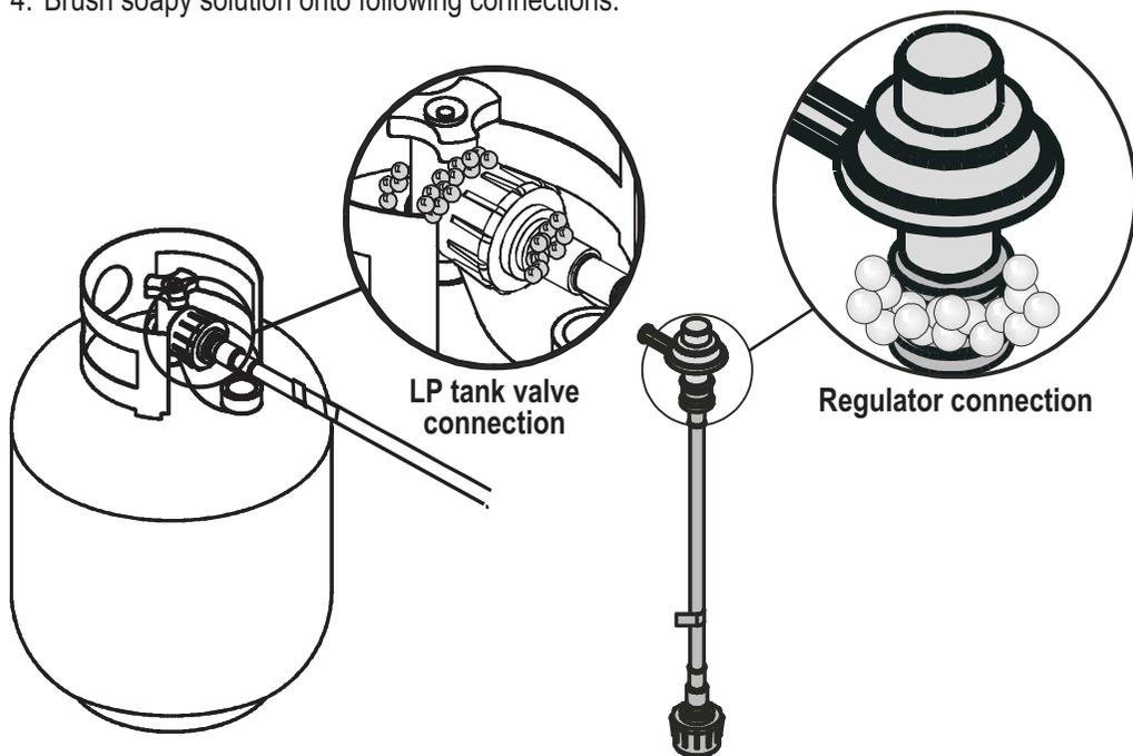
5. **"If growing"** bubbles appear, there is a leak. Close LP tank valve immediately and retighten connections. **If leaks cannot be stopped "do not try to repair"**. Call for replacement parts. Order new parts by giving the serial, model number and name of items needed to the Grill Service Center at 1-800-241-7548 U.S. or 1-800-387-6057 CAN.
