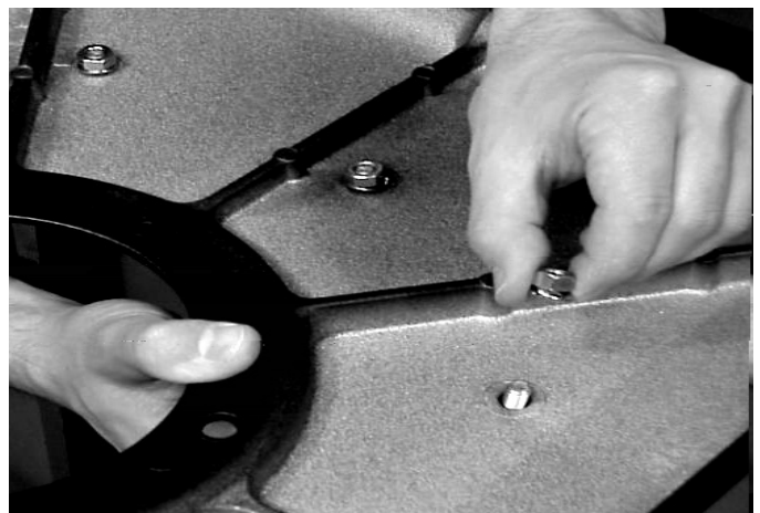
Figure 3 Attaching Pedestal to Base
