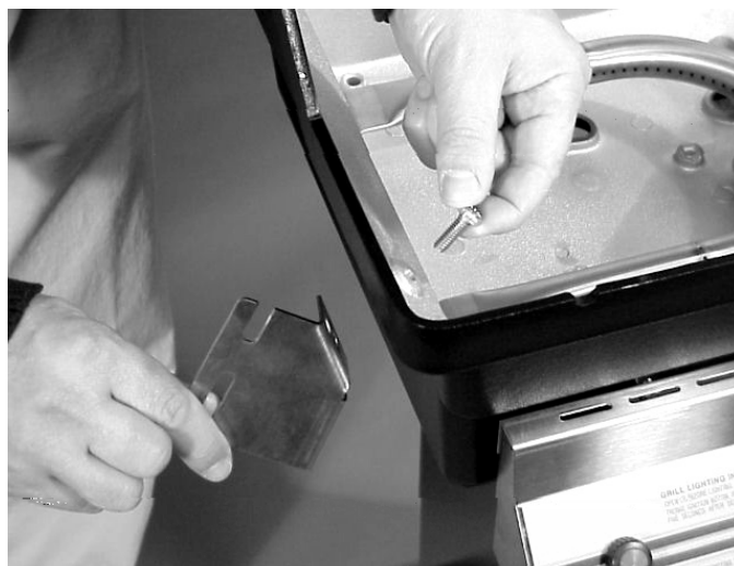
Figure 9 Installing Shelf Bracket
