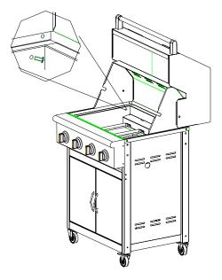
Step 6: Assemble side burner with 8pcs truss head  $\frac{1}{4}$ -20 x  $\frac{1}{2}$ " screws. Align the holes on the right side of grill housing and screw through the holes in the right side shelf and tighten into the grill housing as per the diagram below. Then tighten the gas hose to side burner valve. Repeat this step for the left side shelf.
