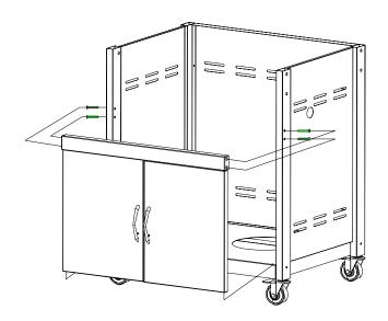
Step 4: Remove the upper portion of grill from carton. Slide-in the upper portion of the grill onto the cart from the front.
