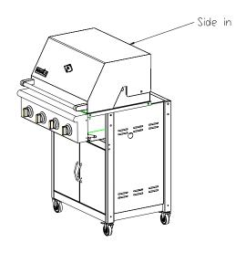
Step 5: Screw the upper portion of the grill to the cart with Truss head  $\frac{1}{4}$ -20 x  $\frac{1}{2}$ ". Screw in four corners of the grill housing. Make sure the four screws are tight.
