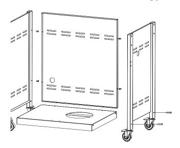
**Step 3:** Align the 2 doors bottom panel hole first & align with cross bar & with top of the 2 sides. Use the four pieces 1/4"-20X1 1/2" screws for the side panel.
