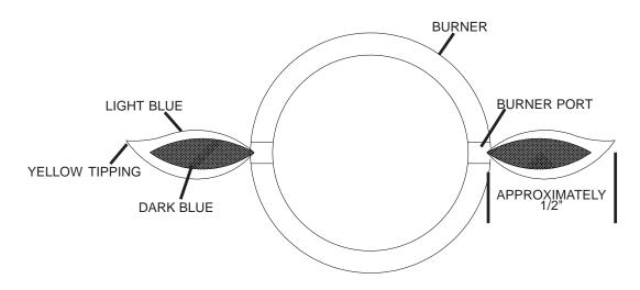
If the burner is getting too little air, the flames will be lazy yellow, and possibly produce soot. If the burner is getting too much air, the flames will be lifting erratically from the burner and may cause difficulties when lighting.
