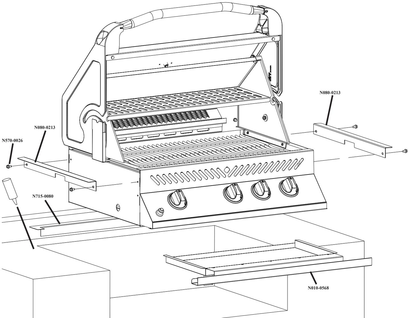
This grill is designed for **MASONRY, NON-COMBUSTIBLE** enclosures only, and must be installed and serviced by a qualified installer to local codes.
