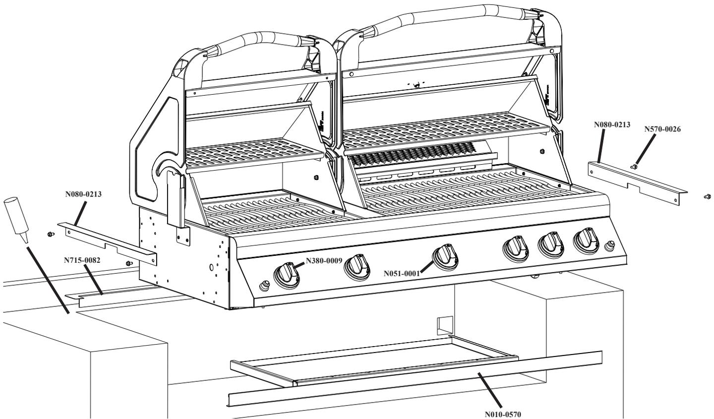
This grill is designed for **MASONRY, NON-COMBUSTIBLE** enclosures only, and must be installed and serviced by a qualified installer to local codes.
