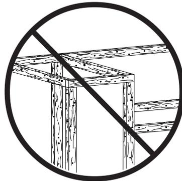
**CABINET FRAME AND CABINET MUST BE MADE FROM NON-COMBUSTIBLE MATERIAL**
