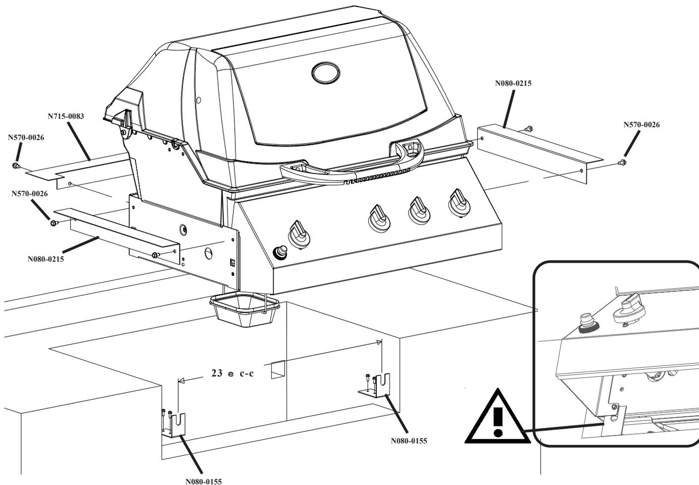
This grill is designed for **MASONRY, NON-COMBUSTIBLE** enclosures only, and must be installed and serviced by a qualified installer to local codes. Access must be provided in the enclosure for drip tray removal and cleaning.
