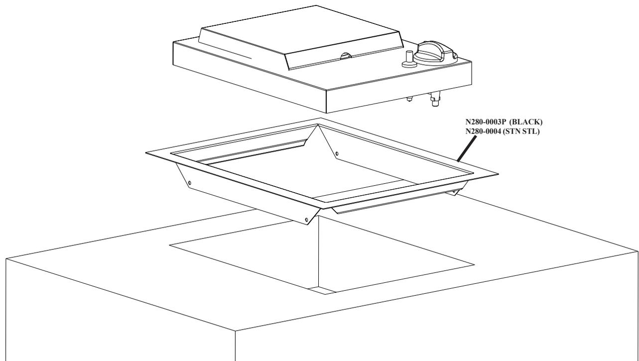
1. Fit the side burner frame into the opening. The frame should be attached to the opening to prevent any future movement (fasteners not included).
