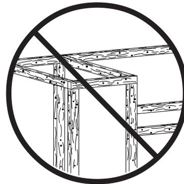
**LA CHARPENTE DU CABINET ET LE CABINET DOIVENT ÊTRE FAITS DE MATÉRIAUX INCOMBUSTIBLES**
