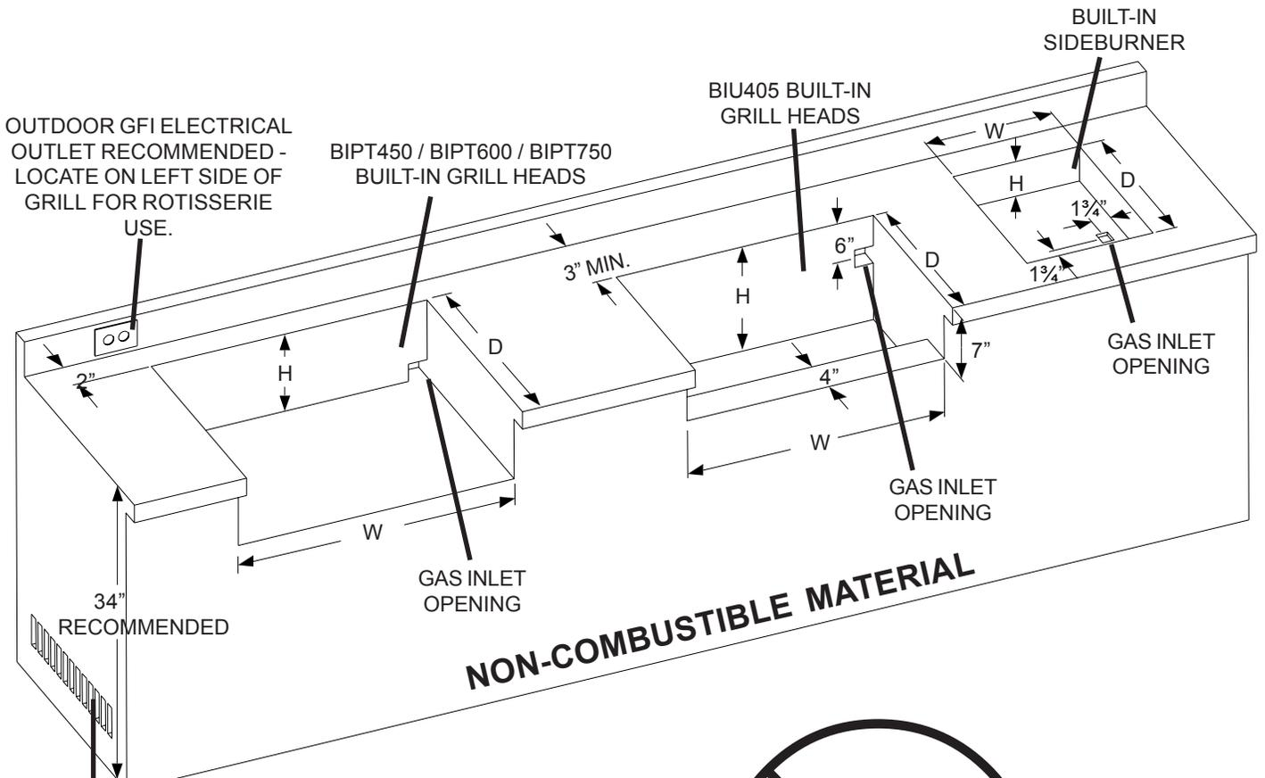
MINIMUM 10 SQ IN OF VENTILATION REQUIRED ON EACH END OF CABINET
