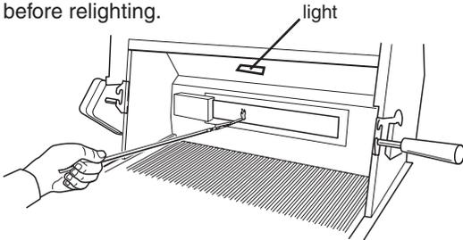
7. Remove the match and replace the manual lighting extension inside the drip tray.
