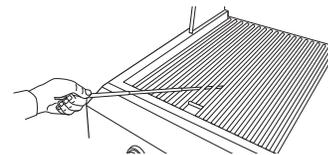
6. Push in and turn the burner knob to “LITE/HI” for the burner closest to the lit match. The burner will light immediately. When burner is lit, turn knob to desired setting.
