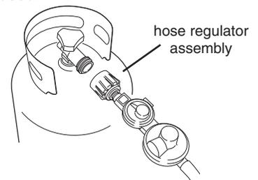
3. Test all connections by brushing on an approved noncorrosive leak-detection solution. Bubbles will show a leak. Correct any leak found.
