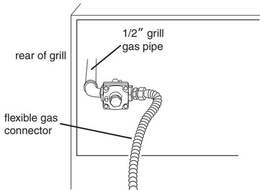
The supply line shall be equipped with an approved shutoff valve. This valve should be located in the same area as the grill and should be in a location that allows ease of opening and closing. Do not block access to the shutoff valve. The valve is for turning on or shutting off gas to the appliance.
