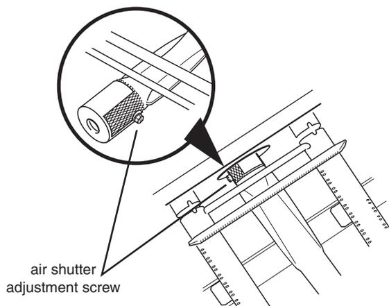
6. Tighten air shutter adjustment screw.
