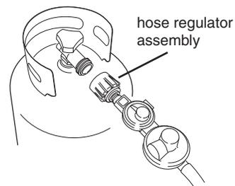
1. Turn on the gas supply. Wait a few minutes for gas to move through the gas line.
