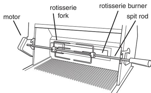
**IMPORTANT:** On Model KFGR383SSS remove the handle from the spit rod when using the side burner. The handle will get "HOT" and failure to remove it will cause the handle to crack and melt.
