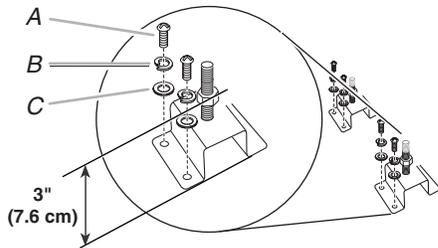
A. Screw (Use proper screw for island floor material.)
