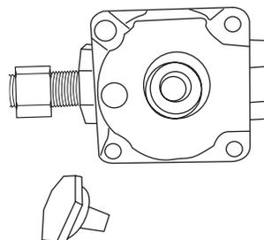
11. Examine the stem on the brass cap. The letters "NAT" should be showing on the end of the plastic stem farthest away from the brass cap.
