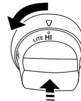
**IMPORTANT:** If the rotisserie burner does not light immediately, turn the rotisserie burner control knob to "OFF" and wait 5 minutes before relighting.
