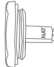
12. Reinstall cap onto convertible regulator.
