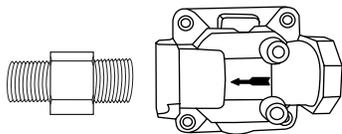
9. Use pipe wrench to install the convertible regulator. Brass cap will be facing up when tight.
