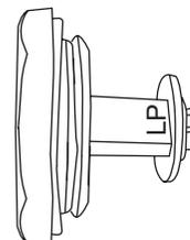
13. Use adjustable wrench to reinstall cap onto regulator.
