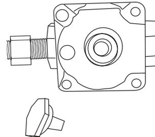
11. Examine the stem on the brass cap. If the letters "NAT" are not showing on the end of the plastic stem farthest away from the brass cap, remove stem from cap, turn it over and snap stem back into the cap so the letters "NAT" are at the end of the stem farthest away from the brass cap.
