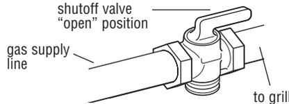
The supply line shall be equipped with an approved shutoff valve. This valve should be located in the same area as the grill and should be in a location that allows ease of opening and closing. Do not block access to the shutoff valve. The valve is for turning on or shutting off gas to the appliance.
