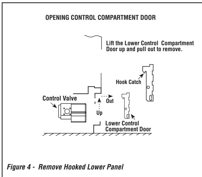
**Figure 4 - Remove Hooked Lower Panel**
