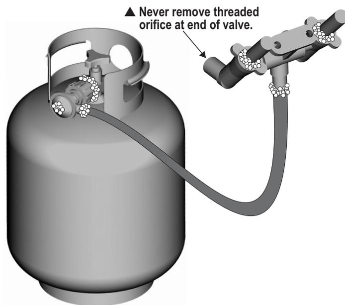
5. If “growing” bubbles appear, there is a leak. Close LP tank valve immediately and retighten connections. **If leaks cannot be stopped do not try to repair.** Call Sears for replacement parts at **1-800-4-MY-HOME®**.
