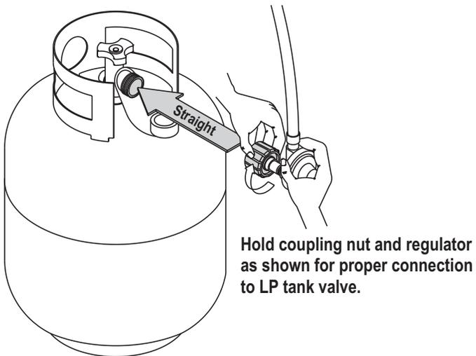
Hold coupling nut and regulator as shown for proper connection to LP tank valve.
