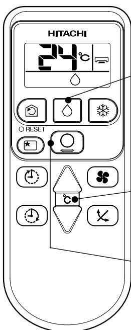
Press the button so that the display indicates (DEHUMIDIFY).
