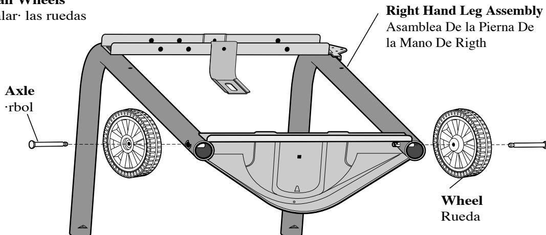
**Place Axle Through Wheel Center. Push Axle into Clip**
