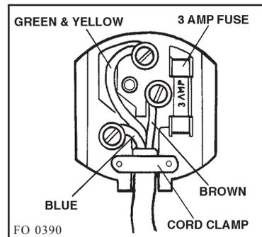
Upon completion there must be no cut, or stray strands of wire present and the cord clamp must be secure over the outer sheath.
