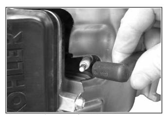
Figure 8-1. Disconnect Spark Plug Leads.
