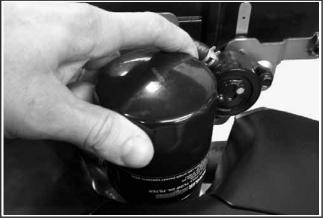
Figure 10-110. Installing and Tightening Oil Filter.
