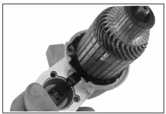
Figure 7-40. Installing Armature and Pivot Lever.
