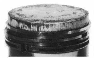
Overheated or Deteriorated Oil
