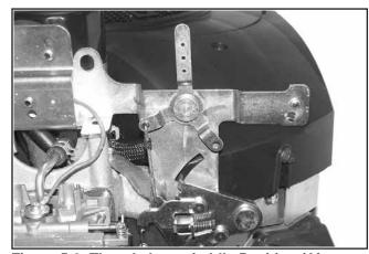
Figure 5-9. Throttle Lever in Idle Position (Air Cleaner Removed for Clarity).
