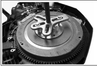
Figure 8-32. Removing Flywheel with a Puller.
