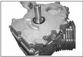
Figure 8-50. Removing Oil Pan Screws.
