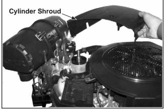
Figure 8-5. Removing Cylinder Shrouds.
