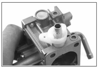
Figure 5-31. Installing Bushing.
