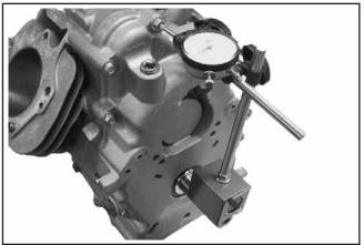
Figure 10-32. Checking Crankshaft End play.
