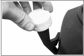
Figure 10-111. Reinstall the Dipstick in Tube.
