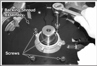
Figure 8-36. Removing Backing Shroud Mounting Screws.
