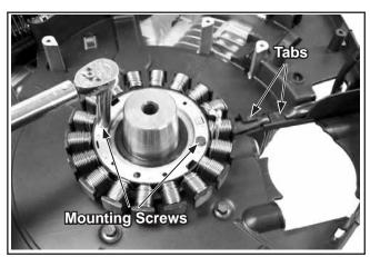
Figure 10-71. Installing Stator.
