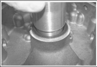
Figure 10-5. Installing Main Bearing.
