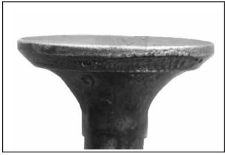
Leakage: A poor grind on face or seat of valve will allow leakage resulting in a burned valve on one side only.
