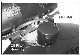
Figure 6-7. Engine Mounted Oil Filter.
