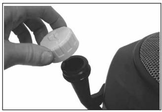
Figure 8-3. Removing Dipstick from Tube.
