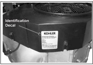
Figure 1-1. Engine Identification Decal Location.
