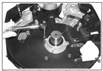
Figure 10-70. Installing Backing Shroud Assembly.
