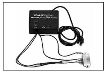
Figure 7-16. Connected Tester.
