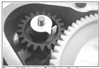
Figure 10-28. Locking Tab Washer Details.
