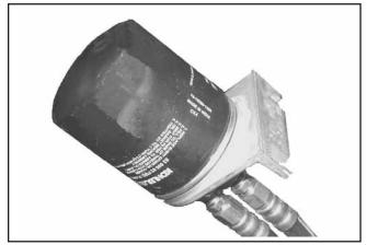
Figure 6-8. Optional Remote Mounted Oil Filter.
