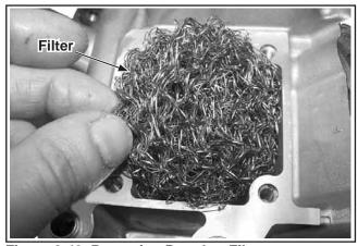
Figure 8-49. Removing Breather Filter.
