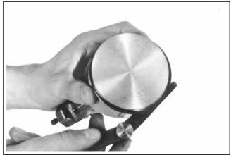
Figure 9-10. Measuring Piston Ring Side Clearance.
