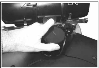
Figure 8-2. Removing Oil Filter.
