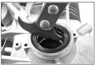
Figure 8-61. Removing Oil Seals.
