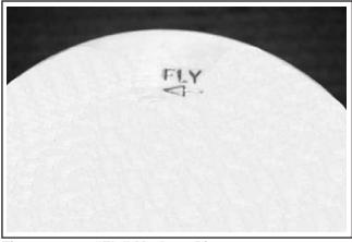
Figure 10-18. "Fly" Mark on Piston.
