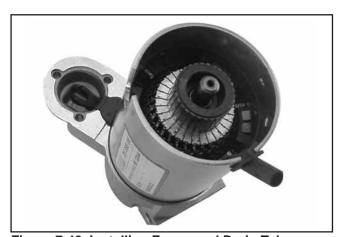
Figure 7-42. Installing Frame and Drain Tube.
