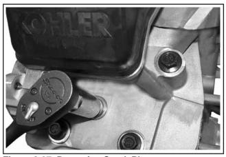
Figure 8-37. Removing Spark Plugs.
