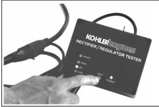
Figure 7-18. Pressing Test Button.
