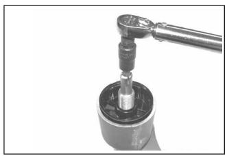
Figure 10-63. Torquing Nipple into Housing.
