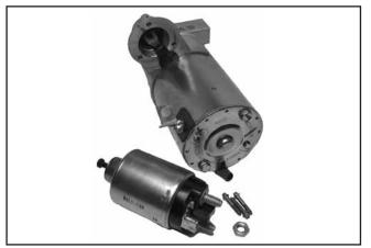
Figure 7-23. Solenoid Removed from Starter.
