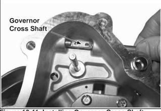
Figure 10-11. Installing Governor Cross Shaft.
