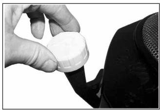
Figure 6-6. Reinstalling Oil Fill Cap/Dipstick.
