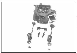
Figure 8-46. Valve Train Components.
