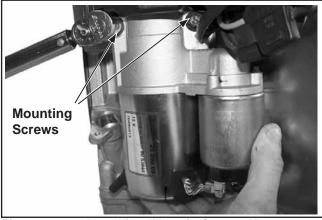
Figure 10-87. Installing Electric Starter Motor.
