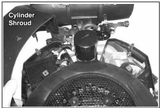
Figure 4-5. Removing Shrouds for Cleaning.
