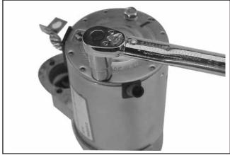
Figure 7-48. Torquing Thru Bolts.
