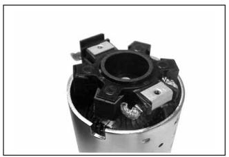
Figure 7-44. Installing Brush Holder Assembly with Supplied Tube.
