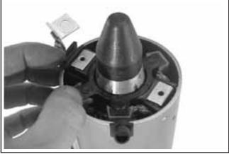
Figure 7-47. Installing Brush Holder Assembly using Tool with Extension.
