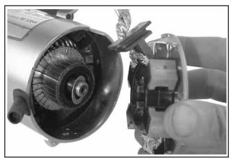
Figure 7-26. Removing Commutator End Plate Assembly.
