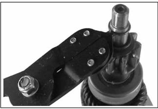
Figure 7-31. Removing Retaining Ring.
