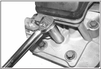
Figure 10-57. Installing Spark Plugs.
