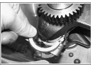
Figure 8-55 Remove Connecting Rod Caps.
