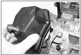
Figure 8-38. Removing Valve Covers.
