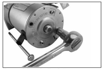
Figure 7-25. Removing Thru Bolts.
