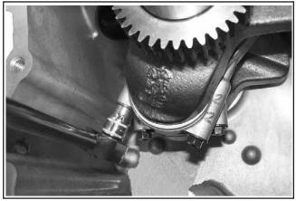
Figure 8-54. Removing Connecting Rod Screws.
