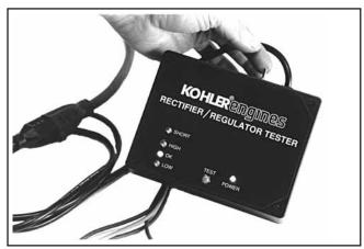
Figure 7-17. Powered Tester.
