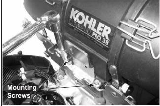
Figure 10-95. Installing Alr Cleaner Mounting Screws.
