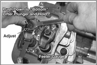
Figure 10-52. Adjusting Valve Clearance.
