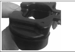
Figure 5-25. Float and Inlet Needle Details.
