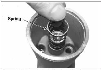
Figure 10-60. Installing Spring into Housing.
