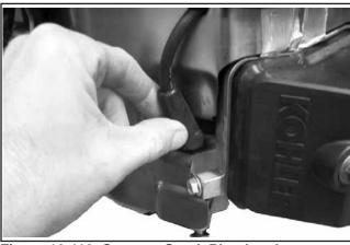
Figure 10-112. Connect Spark Plug Leads.
