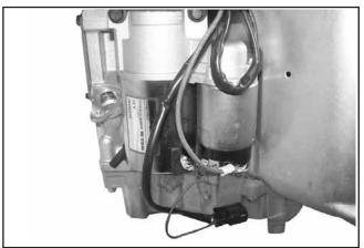
Figure 10-88. Connecting Leads to Starting Motor.
