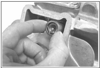
Figure 10-39. Installing Hydraulic Lifters.
