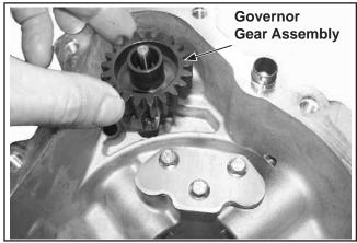
Figure 10-14. Installing Governor Gear Assembly.
