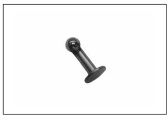
Figure 10-37. Tappet and Ball Bearing Welded Together.
