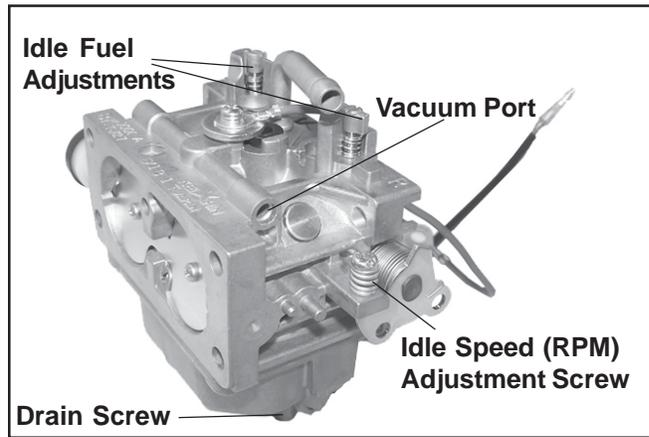
Figure 26. Keihin Two-Barrel Carburetor.
