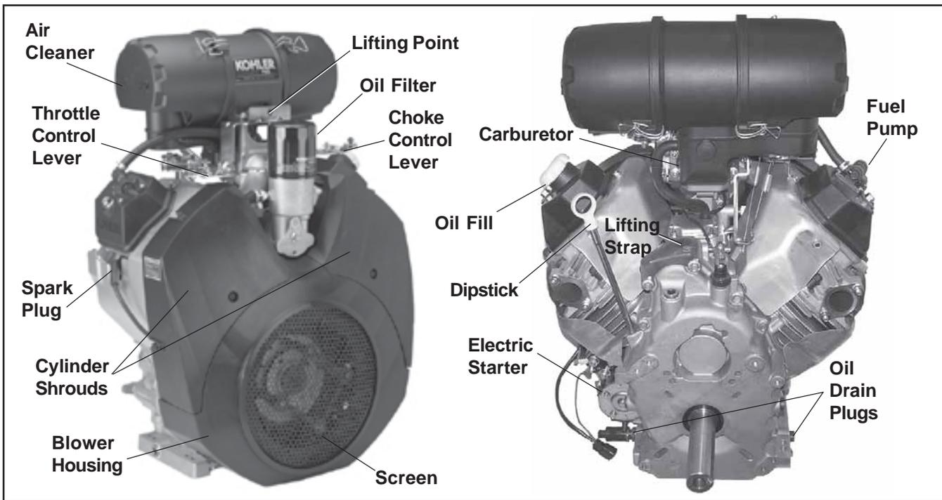
Figure 1. Typical Command PRO Horizontal Shaft Engine.
