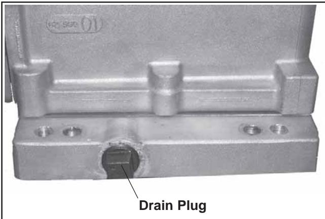
**Figure 13. Oil Drain Plug (No. 2 Side).**
