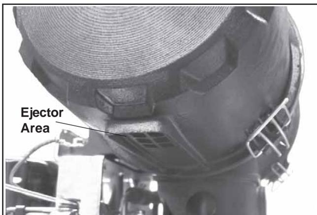
**Figure 22. Ejector Area.**
