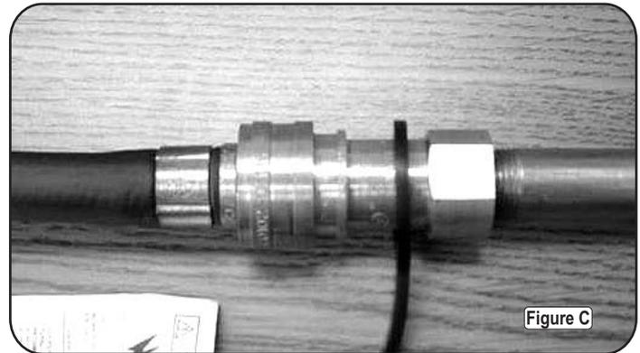
With proper assembly, the gas hose cannot be removed without pushing the quick disconnect sleeve back. To disconnect, push sleeve back and pull plug out of sleeve (this automatically shuts off gas).
