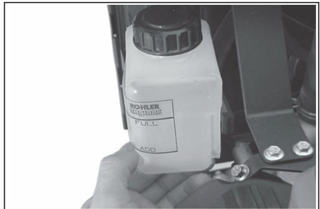
**Figure 13. Removing Reservoir.**
