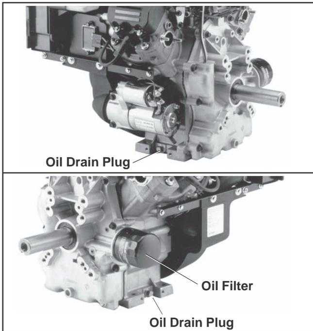
**Figure 8. Oil Drain Plugs and Oil Filter.**
