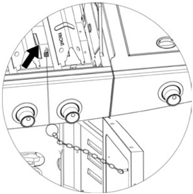
Main Burner Lighting Rod Placement
