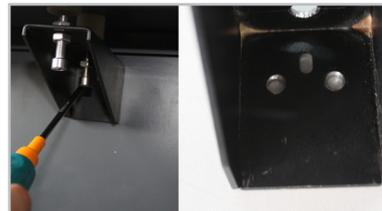
6. Mount the support brackets for the fluorescent lamp fixture (fig. 4.6) to the back side of the upper cross bar with the supplied screws. Insert the fluorescent lamp fixture into the brackets, and insert the fluorescent bulb into the lamp fixture. (fig. 4.6)
