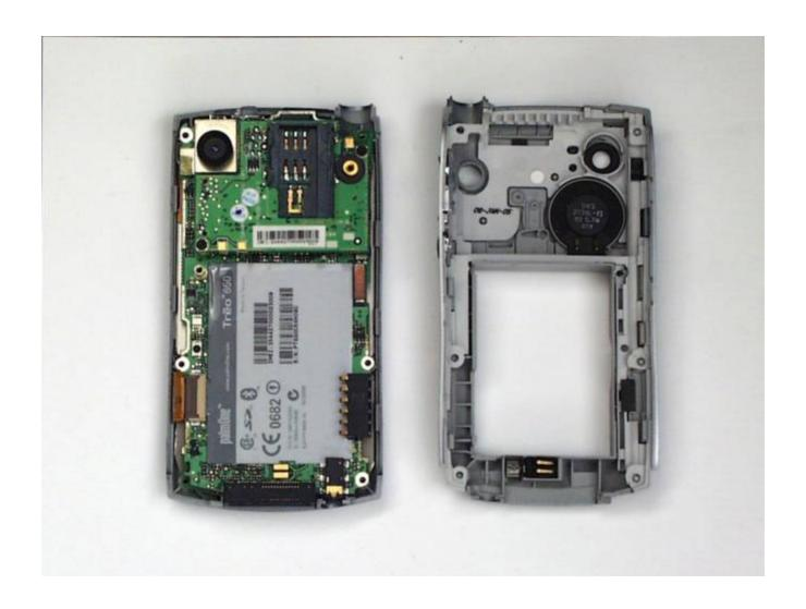
T650.10 REMOVE BUTTON AND VIBRATOR, PRY SPEAKER,
