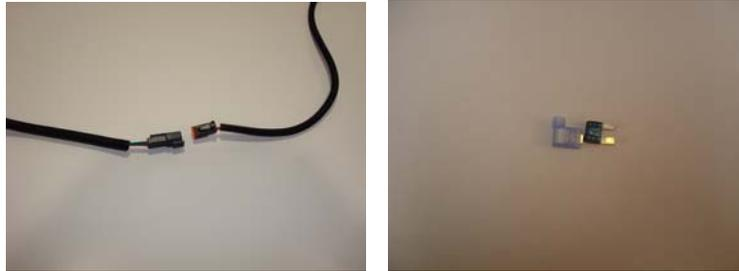
1. Connect the male end of the wire harness to the female electrical connector on the FASS System.
