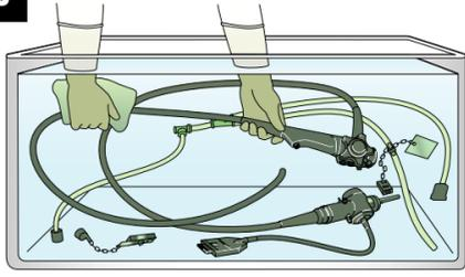
While the endoscope is immersed, disconnect cleaning accessories and use a clean lint-free cloth to wipe away any bubbles clinging to external surfaces.
