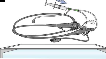
Connect channel plug and injection tube. Inject air to remove disinfectant from air, water and suction channels. Remove endoscope from disinfectant.
