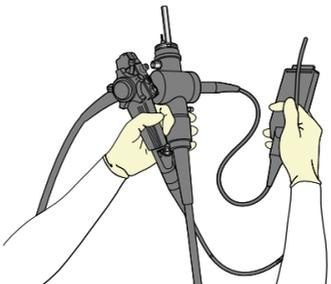
Hold all parts of the endoscope when carrying. Do not let the ends of the endoscope swing freely.
