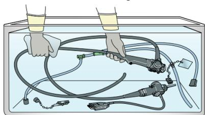
Disconnect channel plug and injection tube. Immerse endoscope and detached parts in water. Thoroughly rinse all external surfaces.
