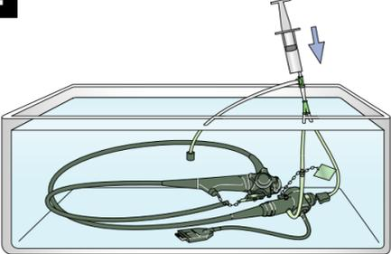
Use syringe to completely fill air, water and suction channels with disinfectant solution.
