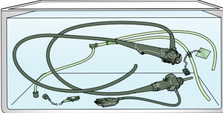
Soak all equipment according to the disinfectant manufacturer's recommended time and temperature. Use a timer to measure exact contact time.
