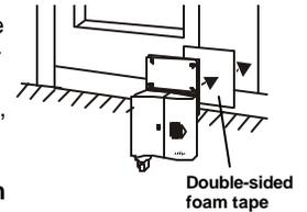
For wooden garage doors, it is recommended to mount the sensor with screws on to the garage door with 3 x 18 screws provided.
