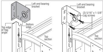
Position the left hand end bearing bracket up against the jamb and the horizontal track, as shown. Fasten the left hand end bearing bracket to the horizontal track with (1) 3/8"-16 x 3/4" truss head bolt and (1) 3/8"-16 nut. Secure the left hand end bearing bracket to the jamb using (3) 5/16" x 1-5/8" lag screws. Repeat same process for the other side.
