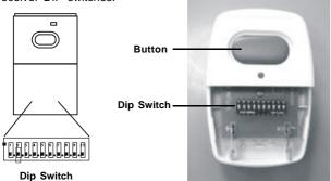
3. Test the transmitter by pressing onto the button (see figure), the red LED should come on and it should activate the garage door. Close the case firmly.
