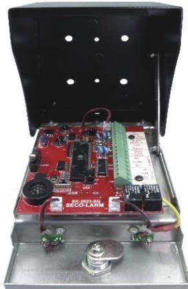
Unique faceplate hinge allows for easy installation.
