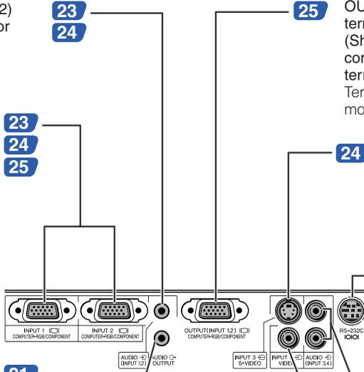
OUTPUT (INPUT 1, 2) terminal (Shared computer RGB and component signals output terminal for INPUT 1 and 2) Terminal for connecting a monitor.
