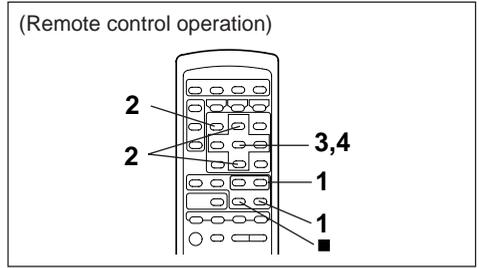
**1** Whilst in the stop mode, select the second of the two adjacent tracks you want to combine pressing the ◀◀◀ or ▶▶▶ button. Or start playing the second of the two tracks you want to combine, and then press the ► || button.
