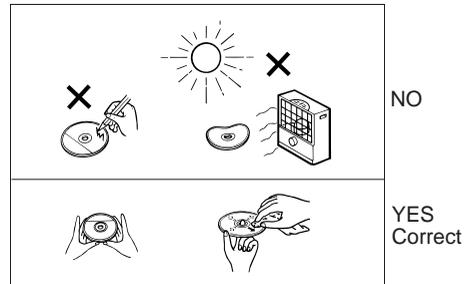
Compact discs are fairly resistant to damage, however mistracking can occur due to an accumulation of dirt on the disc surface.
