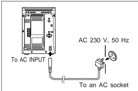
Connect the AC power lead to the AC INPUT socket, then connect the AC power lead plug to an AC socket.
