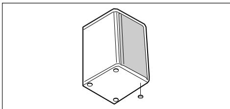
Attach the cushions to the bottom of the speaker to prevent it from sliding.
