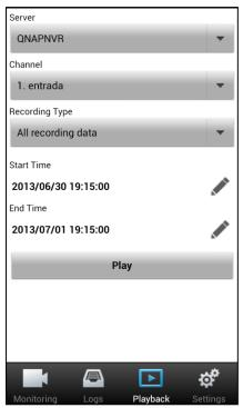
Enter the "Playback" screen to search and playback the recording files on an NVR.
