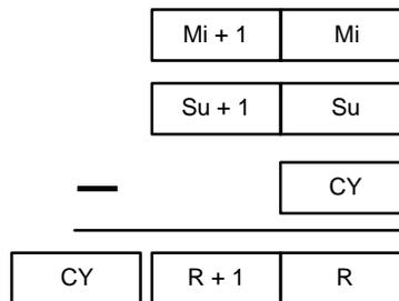
SBBL(—) can also be used to subtract signed binary data. The underflow and overflow flags (SR 25404 and SR 25405) indicate whether the result has exceeded the lower or upper limits of the 32-bit signed binary data range. Refer to page 29 for details on signed binary data.
