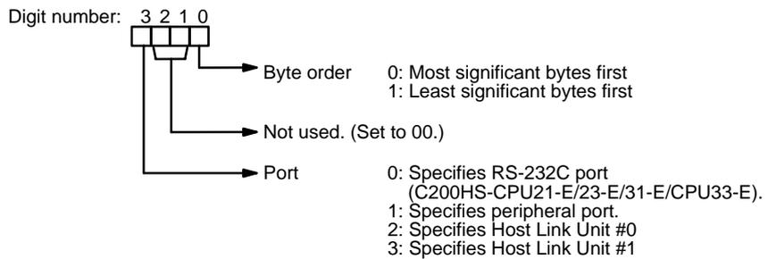
The specified number of bytes will be read from S through S+(N/2)-1, converted to ASCII, and transmitted through the specified port. The bytes of source data shown below will be transmitted in this order: 12345678...
