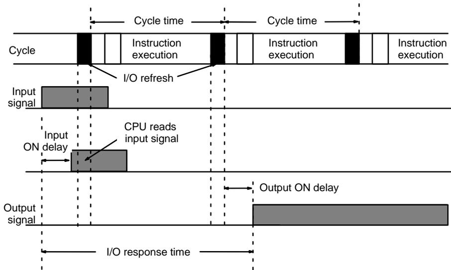
$$\text{Minimum I/O response time} = \text{Input ON delay} + \text{Cycle time} + \text{I/O refresh time} + \text{Output ON delay}$$
