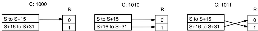
The following is an example of a one-byte encode operation to the rightmost byte of R (C would be 1000 in this case).
