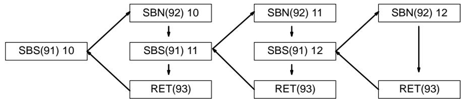
The following diagram illustrates program execution flow for various execution conditions for two SBS(91).
