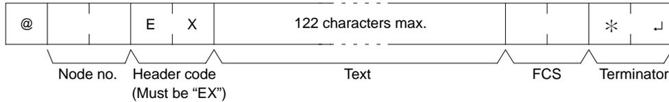
One byte of data (2 digits hexadecimal) is converted to two characters in ASCII for transmission, the amount of data in the transmission is twice the amount of words specified for TXD(—). The maximum number of characters for transmission is 122 and the maximum number of bytes that can be designated for TXD(—) is one half of that, or 61.
