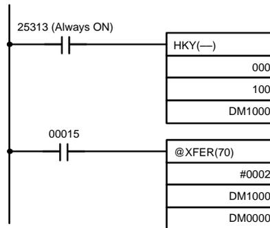
The hexadecimal key information that is input to IR 000 by HKY(—) is converted to hexadecimal and stored in words DM1000 and DM1001.
