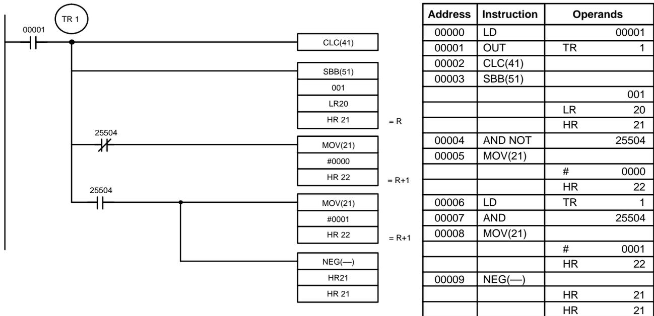
In the case below, the content of LR 20 (#7A03) and CY are subtracted from IR 001 (#F8C5). The result is stored in HR 21 and the content of HR 22 (#0000) indicates that the result is positive.
