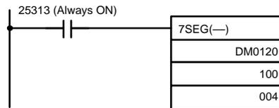
The 8-digit BCD data in DM 0120 (rightmost 4 digits) and DM 0121 (leftmost 4 digits) are always displayed by means of 7SEG(—). When the contents of DM 0120 and DM 0121 change, the display will also change.
