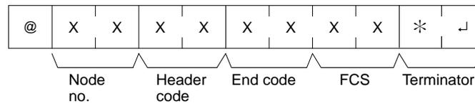
The header code will vary according to the command and can contain a subcode (for composite commands).
