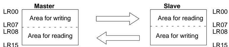
When the program is executed at both the master and the slave, the status of IR 001 of each Unit will be reflected in IR 100 of the other Unit. IR 001 is an input word and IR 100 is an output word.
