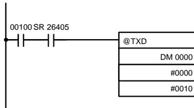
If SR 26405 (the Transmit Ready Flag) is ON when IR 00100 turns ON, the ten bytes of data (DM 0000 to DM 0004) will be transmitted.
