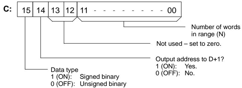
**Caution** If bit 14 of C is ON, values above #8000 are treated as negative numbers, so the results will differ depending on the specified data type. Be sure that the correct data type is specified.
