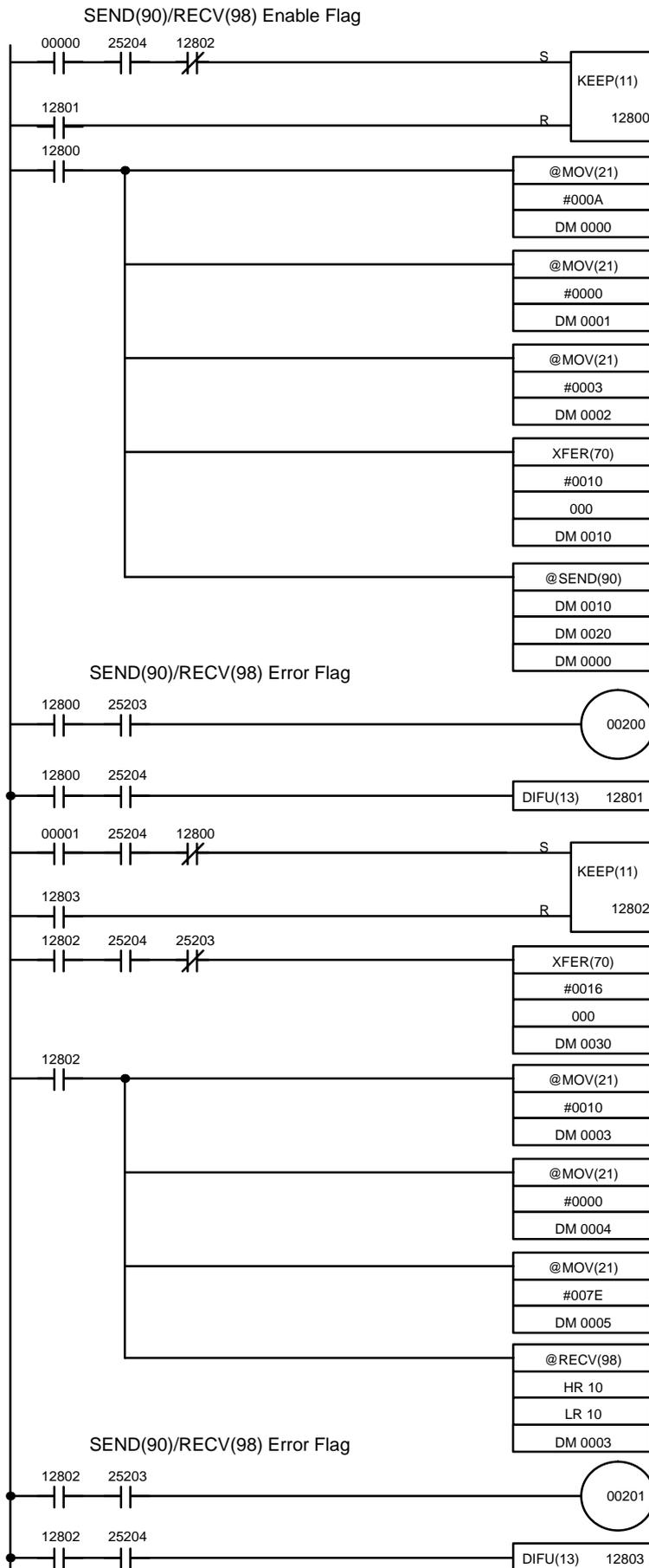
12800 prevents execution of SEND(90) until RCV(98) (below) has completed. IR 00000 is turned ON to start transmission.
