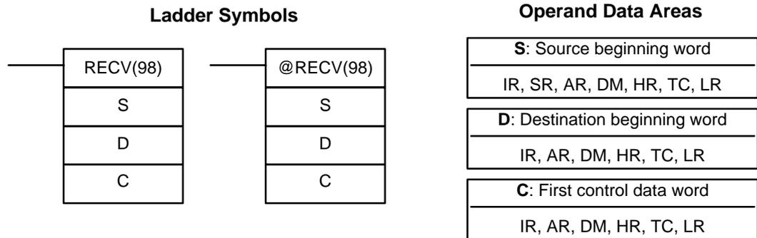
**Limitations** Can be performed with the CPU31-E/33-E only. C through C+2 must be within the same data area and must be within the values specified below. To be able to use RECV(98), the system must have a SYSMAC NET Link or SYSMAC LINK Unit mounted.
