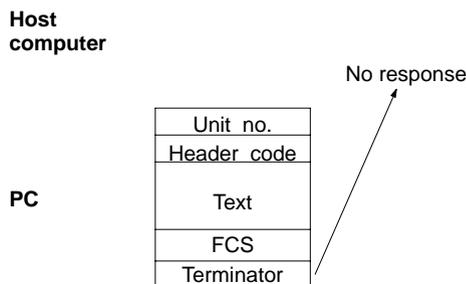
When commands are issued to the host computer, the data is transmitted in one direction from the PC to the host computer. If a response to a command is required use a host link communications command to write the response from the host computer to the PC.
