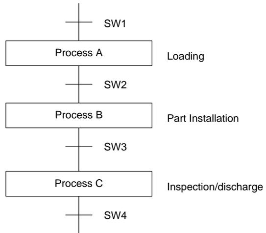
The program for this process, shown below, utilizes the most basic type of step programming: each step is completed by a unique SNXT(09) that starts the next step. Each step starts when the switch that indicates the previous step has been completed turns ON.
