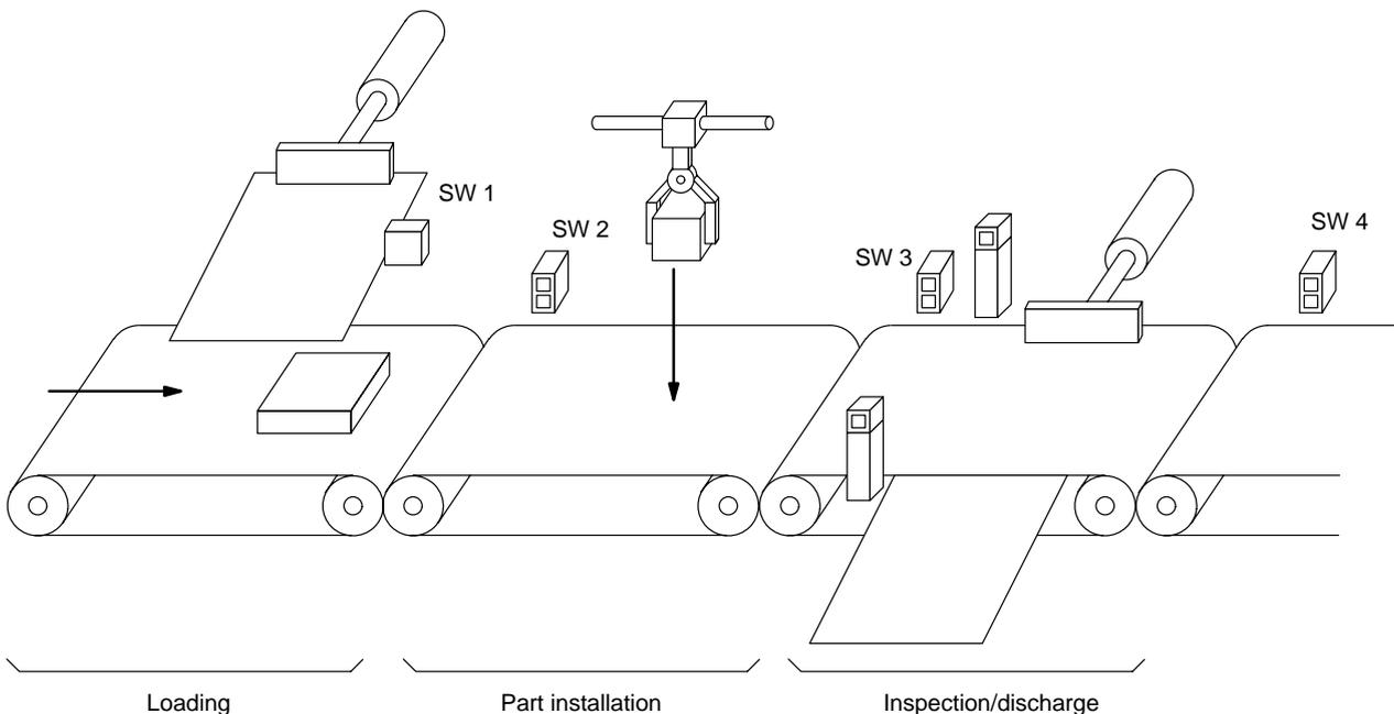
The following diagram demonstrates the flow of processing and the switches that are used for execution control.
