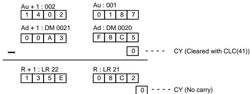
**Note** The status of the UF and OF flags can be ignored since they are relevant only in the subtraction of signed binary data.
