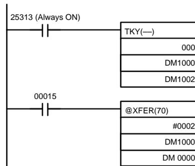
The 10-key information input to IR 000 using TKY(—) is converted to BCD and stored in DM 1000 and DM 1001. Key information is stored in DM 1002.
