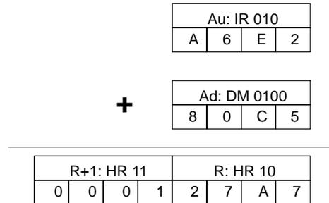
**Note** The UF and OF flags would also be turned ON during this addition, but they can be ignored since they are relevant only in the addition of signed binary data.
