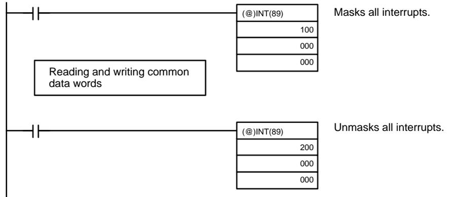
Data concurrence can also be a problem if interrupts occur during data transfers occurring in servicing for Special I/O Units, remote I/O, or Host Link Systems. For any of these, data can be non-concurrent down to byte units.
