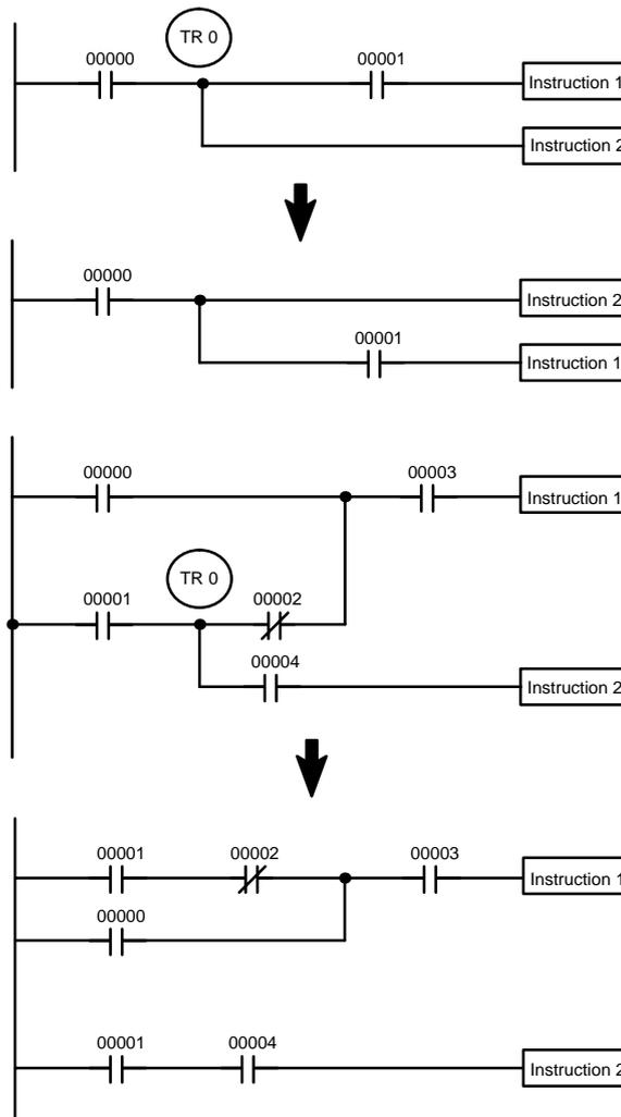
**Note** TR bits are only used when programming using mnemonic code. They are not necessary when inputting ladder diagrams directly. The above limitations on the number of branching points requiring TR bits, and considerations on methods to reduce the number of programming instructions, still hold.
