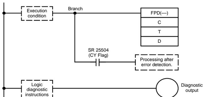
When the execution condition is OFF, FPD(—) is not executed. When the execution condition is ON, FPD(—) monitors the time until the logic diagnostics condition goes ON, turning ON the diagnostic output. If this time exceeds T, the following will occur:
