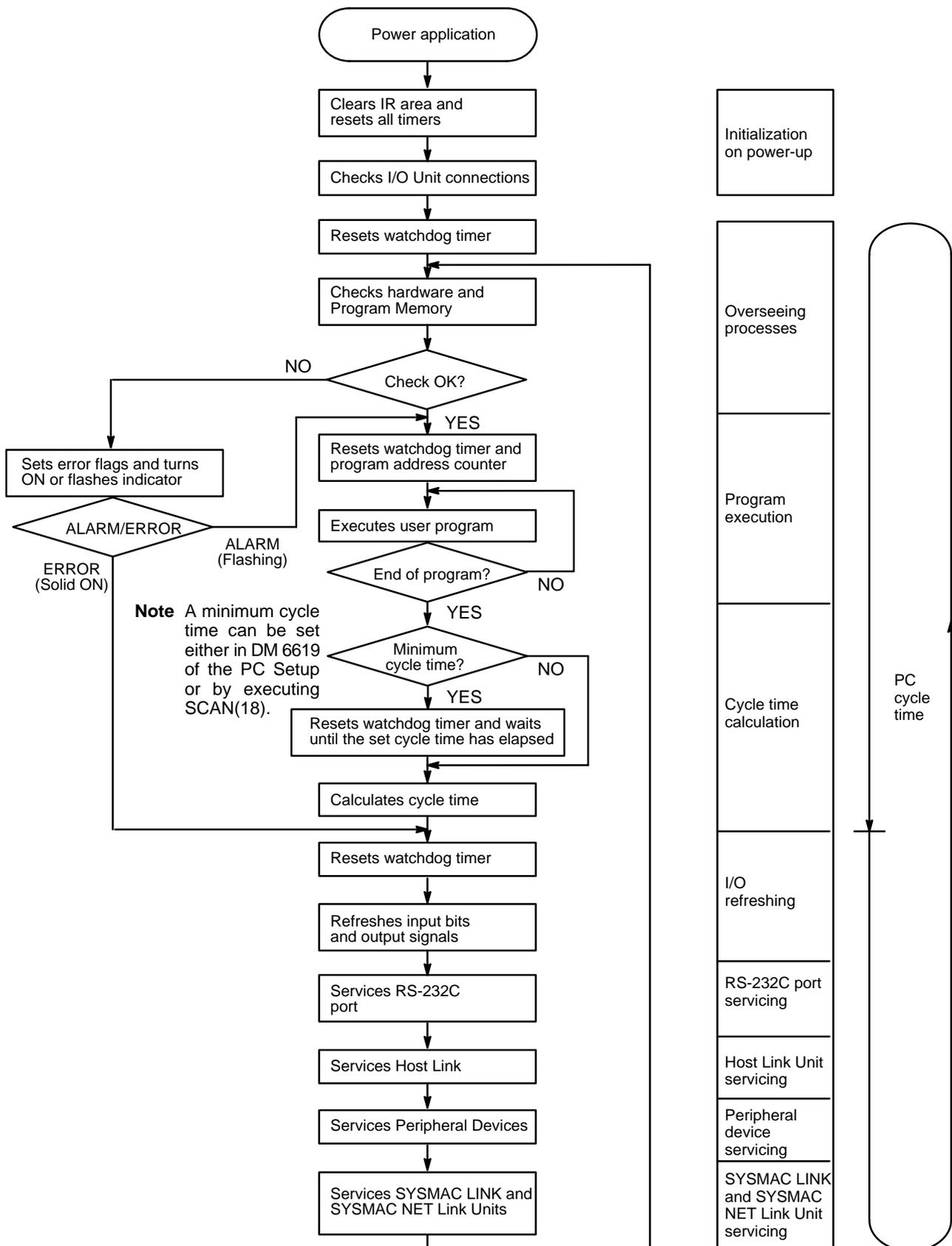
The first three operations immediately after power application are performed only once each time the PC is turned on. The rest of the operations are performed in cyclic fashion. The cycle time is the time that is required for the CPU to complete one of these cycles. This cycle includes basically eight types of operation.
