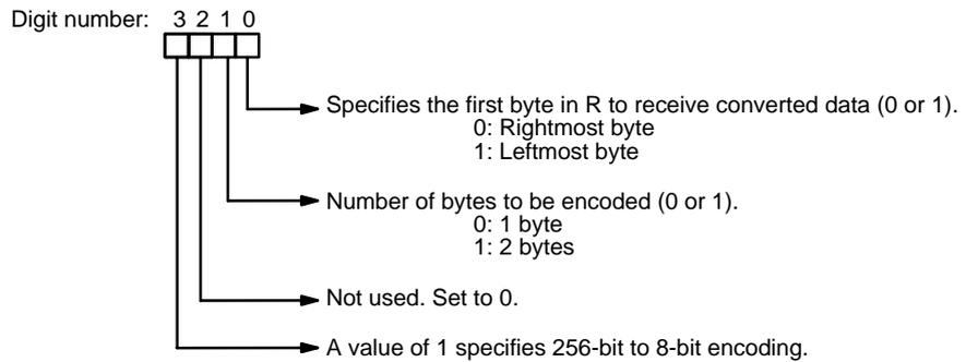
Three possible C values and the conversions that they produce are shown below. (In R, 0 indicates the rightmost byte and 1 indicates the leftmost byte.)
