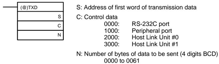
3. From the time this instruction is executed until the data transmission is complete, SR 26405, SR 26413, SR 26705, or SR 26713 will remain OFF. The bits for the RS-232C or peripheral port will turn ON again upon completion of the data transmission. The bits for the Host Link Units will turn ON again when the data transmission has been passed to the Host Link Unit.
