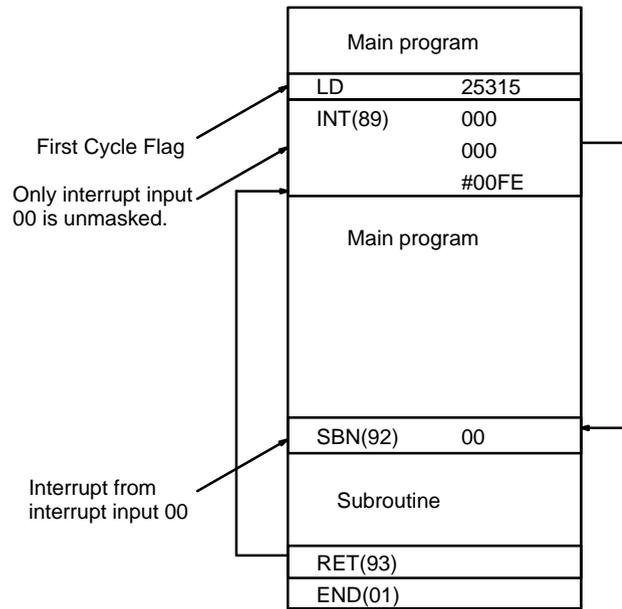
**Note** Depending on the setting of DM 6621 in the PC Setup, Host Link servicing, Remote I/O servicing, Special I/O Unit servicing, and individual instruction execution will be completed before the subroutine is executed. Refer to page 255 for details.
