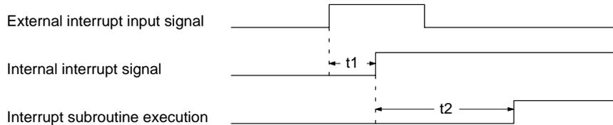
t1 = ON delay of Interrupt Input Unit
