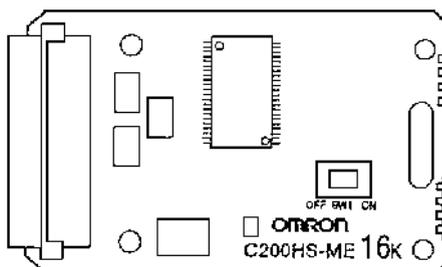
**C200HS-MP□16K (EPROM)** The program is written using a PROM Writer. The ROM is mounted to the Memory Cassette and then installed in the CPU. I/O data cannot be stored.
