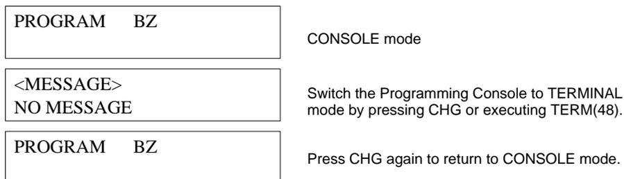
**Expansion TERMINAL Mode** The Programming Console can be put into Expansion TERMINAL mode by turning ON AR 0709. Pin 6 of the CPU's DIP switch must be ON.
