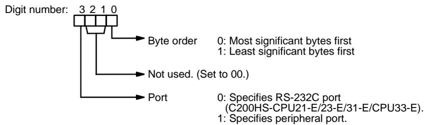
The specified number of bytes will be read from S through S+(NP2)-1 and transmitted through the specified port.
