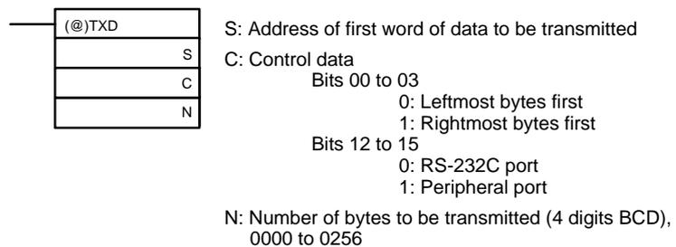
3. From the time this instruction is executed until the data transmission is complete, SR 26405 (or SR 25413 for the peripheral port) will remain OFF. It will turn ON again upon completion of the data transmission.
