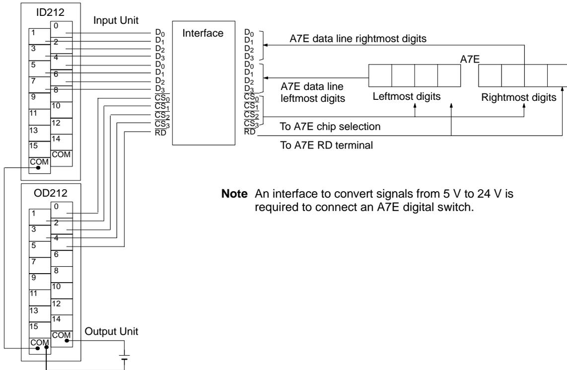
**Note** An interface to convert signals from 5 V to 24 V is required to connect an A7E digital switch.
