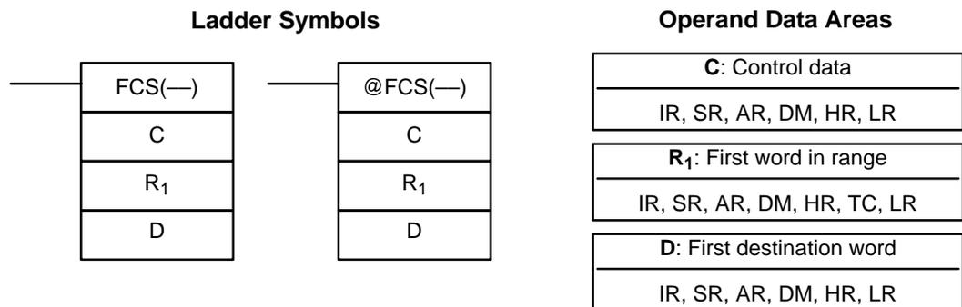
**Description** FCS(—) can be used to check for errors when transferring data through communications ports.
