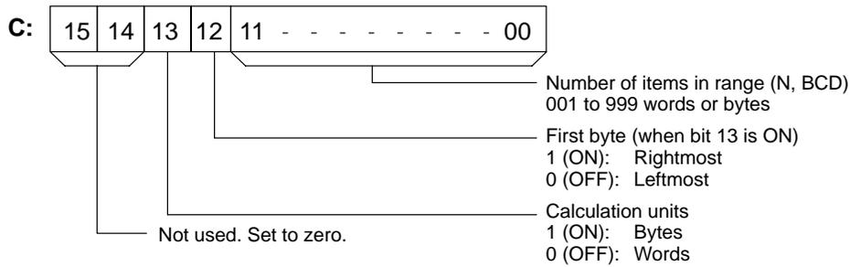
**Number of Items in Range** The number of items within the range (N) is contained in the 3 rightmost digits of C, which must be BCD between 001 and 999.
