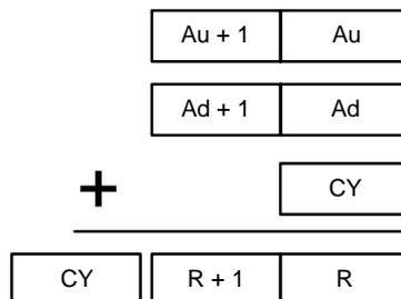
ADBL(—) can also be used to add signed binary data. The underflow and overflow flags (SR 25404 and SR 25405) indicate whether the result has exceeded the lower or upper limits of the 32-bit signed binary data range. Refer to page 29 for details on signed binary data.
