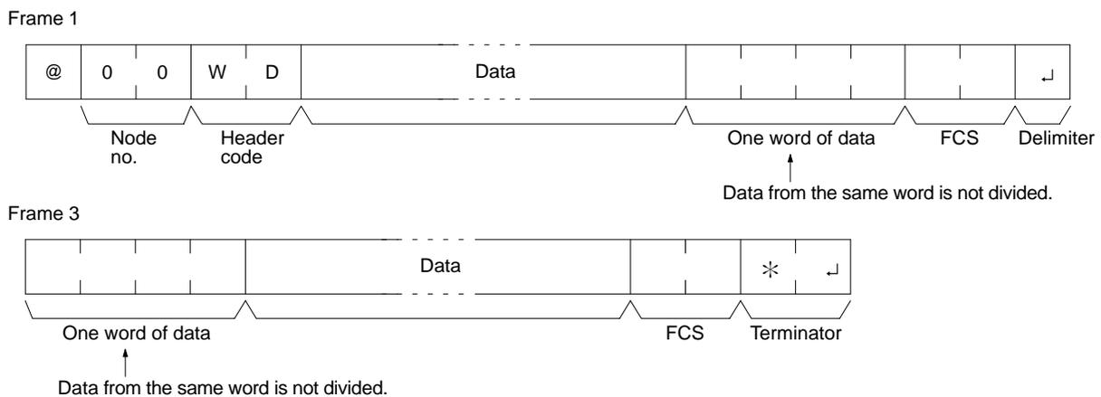
**FCS (Frame Check Sequence)** When a frame is transmitted, an FCS is placed just before the delimiter or terminator in order to check whether any data error has been generated. The FCS is 8-bit data converted into two ASCII characters. The 8-bit data is the result of an EXCLUSIVE OR performed on the data from the beginning of the frame until the end of the text in that frame (i.e., just before the FCS). Calculating the FCS each
