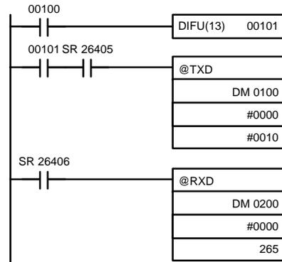
If SR 26405 (the Transmit Ready Flag) is ON when IR 00100 turns ON, the ten bytes of data (DM 0100 to DM 0104) will be transmitted, leftmost bytes first.
