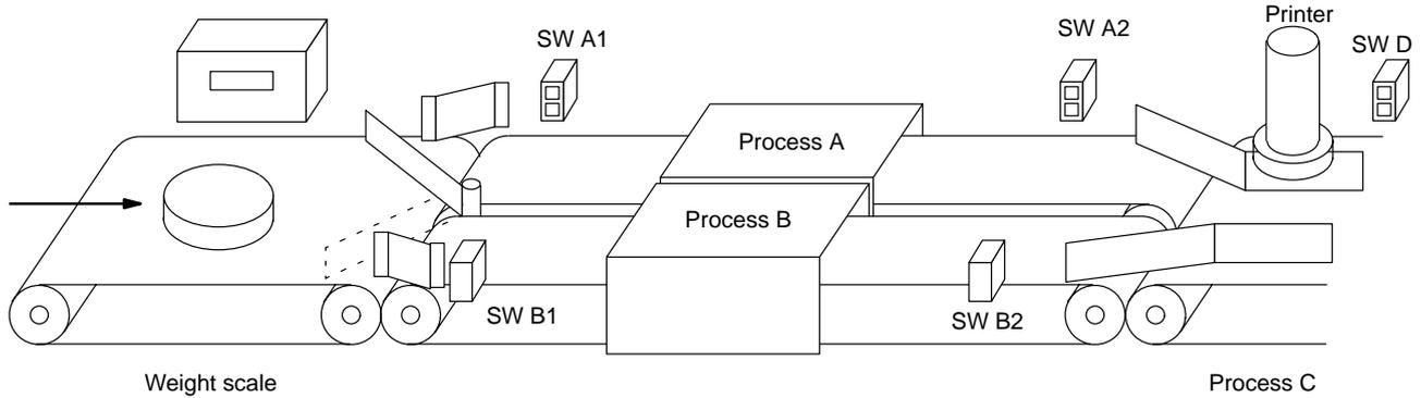
The following diagram demonstrates the flow of processing and the switches that are used for execution control. Here, either process A or process B is used depending on the status of SW A1 and SW B1.
