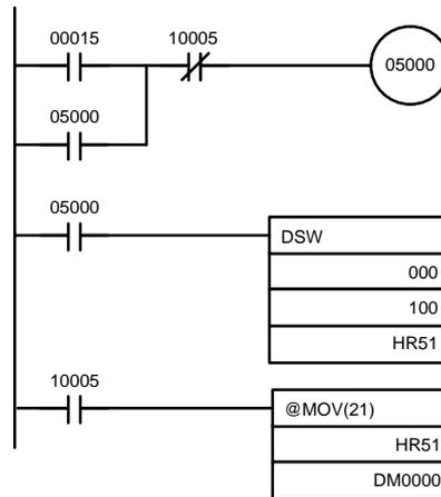
When IR 00015 turns ON, the IR 05000 will hold itself ON until the One Round Flag (IR 10005) turns ON upon completion of one round of reading by DSW(—). The data set from the digital switch by DSW(—) is stored in HR 51. When the One Round Flag (10005) turns ON after reading has been completed, the number stored in HR 51 is transferred to DM 0000.
