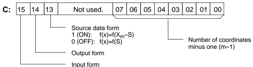
Enter the coordinates of the m+1 end-points, which define the m line segments, as shown in the following table. Enter all coordinates in BIN form. Always enter the coordinates from the lowest X value (X<sub>1</sub>) to the highest (X<sub>m</sub>). X<sub>0</sub> is 0000, and does not have to be entered.
