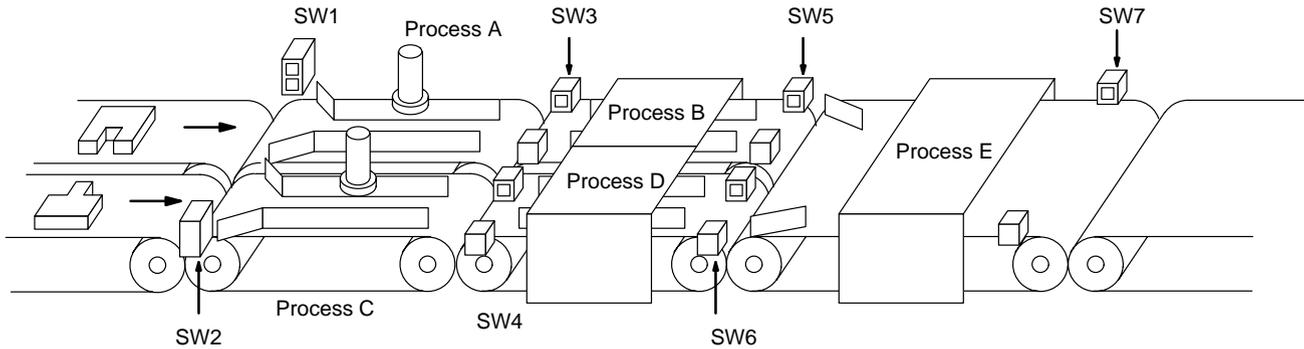
The following diagram demonstrates the flow of processing and the switches that are used for execution control. Here, process A and process C are started together. When process A finishes, process B starts; when process C finishes, process D starts. When both processes B and D have finished, process E starts.
