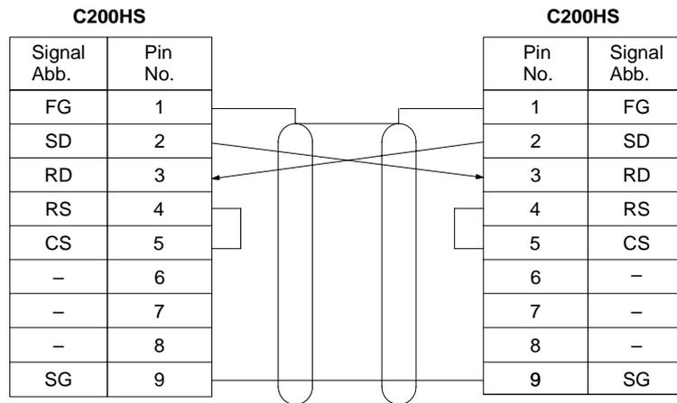
**Note** Ground the FG terminals the C200HS to a resistance of 100 Ω or less.
