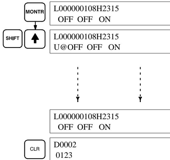
Monitor the desired bit so that it is leftmost on the screen.
