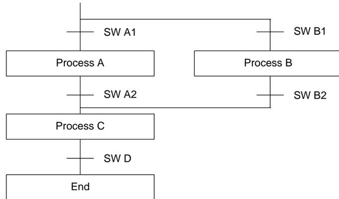
The program for this process, shown below, starts with two SNXT(09) instructions that start processes A and B. Because of the way 00001 (SW A1) and 00002 (SW B1) are programmed, only one of these will be executed to start either process A or process B. Both of the steps for these processes end with a SNXT(09) that starts the step for process C.
