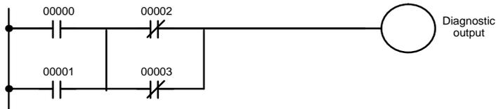
When IR 00000 to IR 00003 are ON, the normally closed condition IR 00002 would be found as the cause of the diagnostic output not turning ON.
