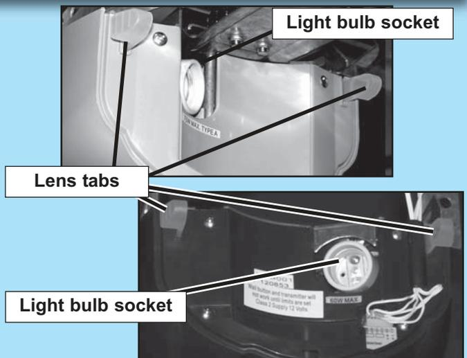
FIG. 9-1 Slide each lens onto motor cover.
