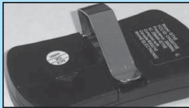
FIG. 8-3 Attach visor clip.
