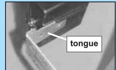
FIG. 3-3 Attaching STB's to brackets.
