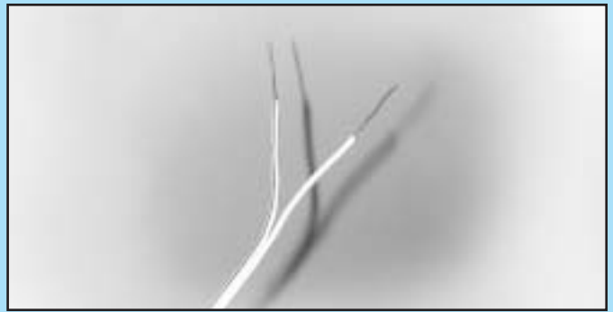
FIG. 3-6 Splitting and stripping.
