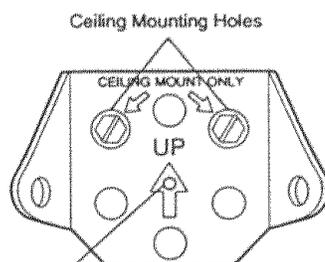
The nail hole is for positioning only. You must use lag screws to mount the header bracket.
